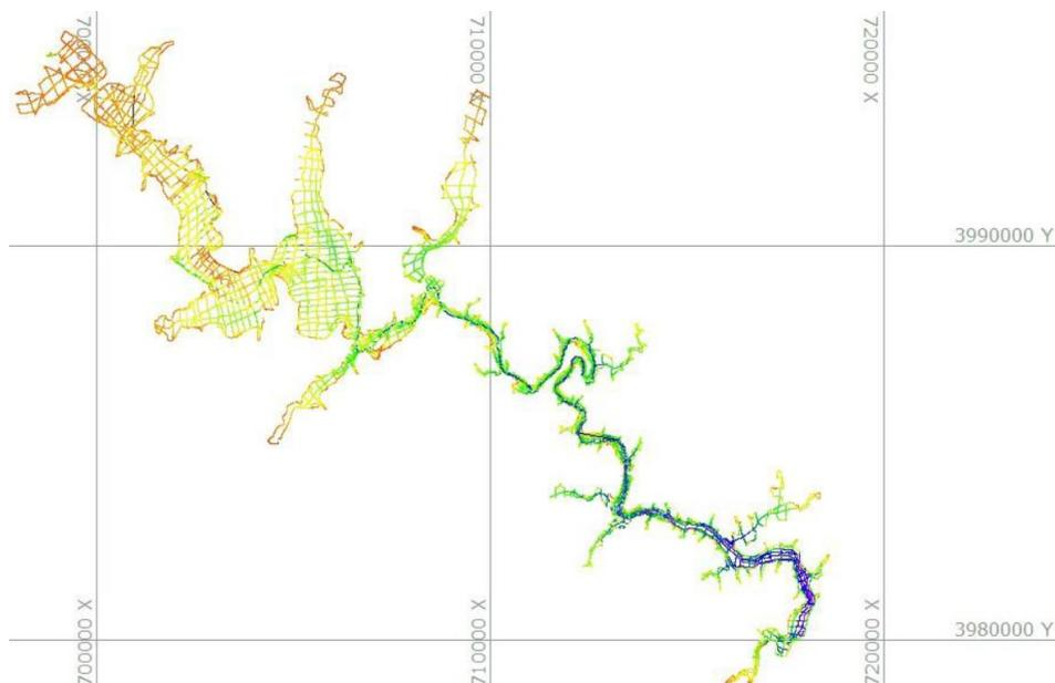
**Figure 5-6. Track line locations for the bathymetric and sediment depth survey**
