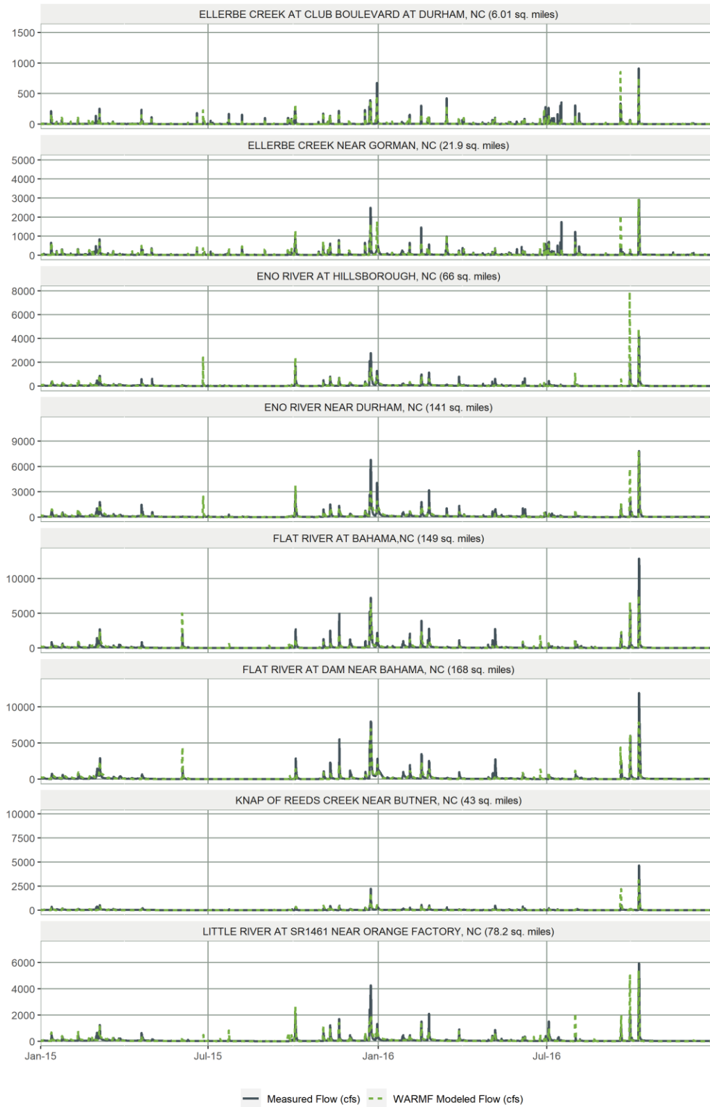
Figure 6-4. Time Series of Simulated and Observed Stream Flows for the Calibration Period (2015 to 2016)
