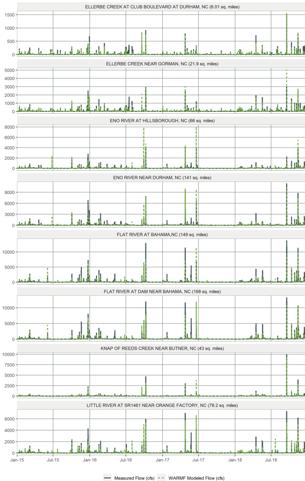
Figure 6-6. Time Series of Simulated and Observed Stream Flows for the Recent Model Period (2015 to 2018)
