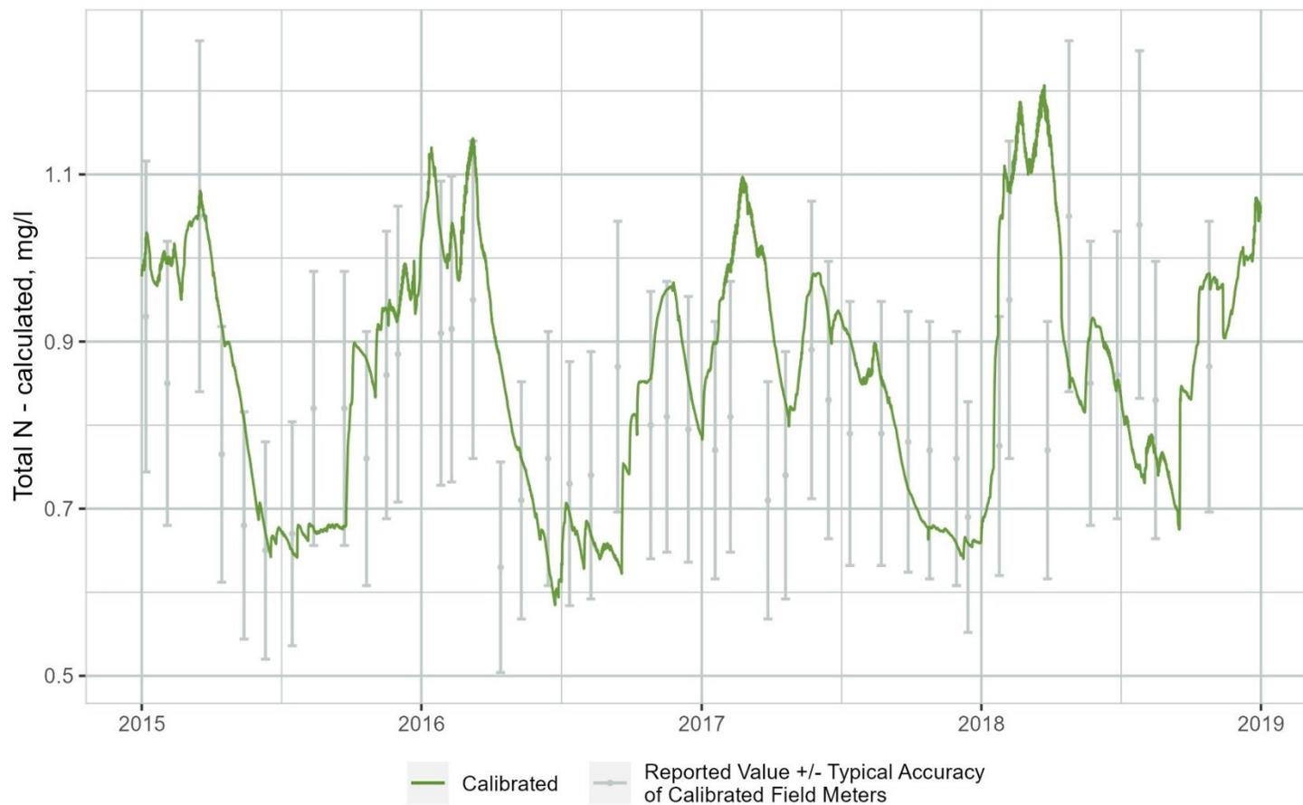
Figure B-35. Time Series Comparison of WARMF Lake Simulated Total Nitrogen (TN) Concentrations to Observations Collected at the Downstream End of Segment 3
