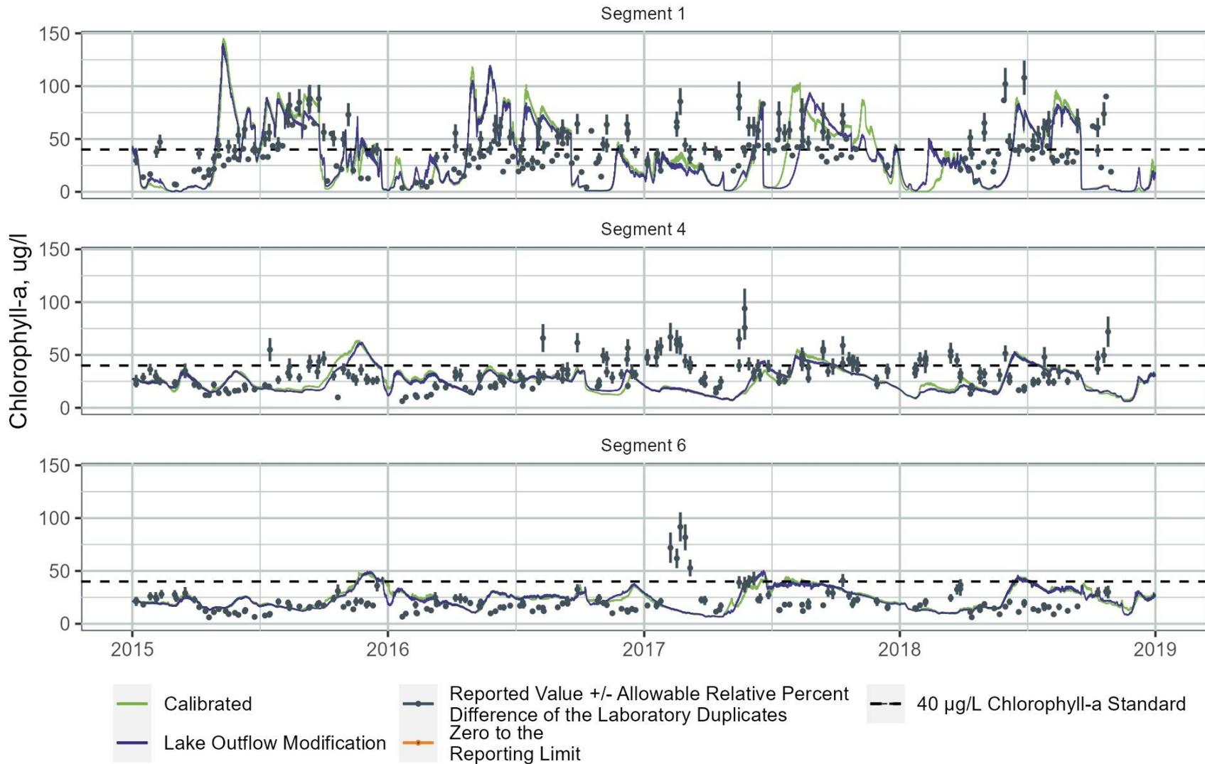
Figure B-118. WARMF Lake Simulated Chlorophyll-a Concentrations for the Calibrated Model Compared to the Dam Release Scenario with the Spillway Elevation Set to Normal Pool in Segment 1 (upper lake near Interstate 85), Segment 4 (middle lake near Highway 50), and Segment 6 (lower lake near the dam)
