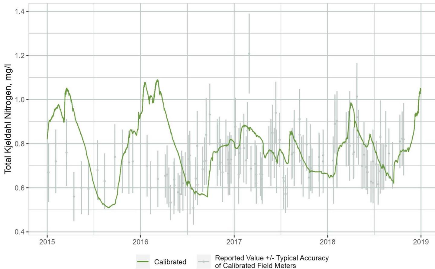
**Figure B-30. Time Series Comparison of WARMF Lake Simulated Total Kjeldahl Nitrogen (TKN) Concentrations to Observations Collected at the Downstream End of Segment 4**
