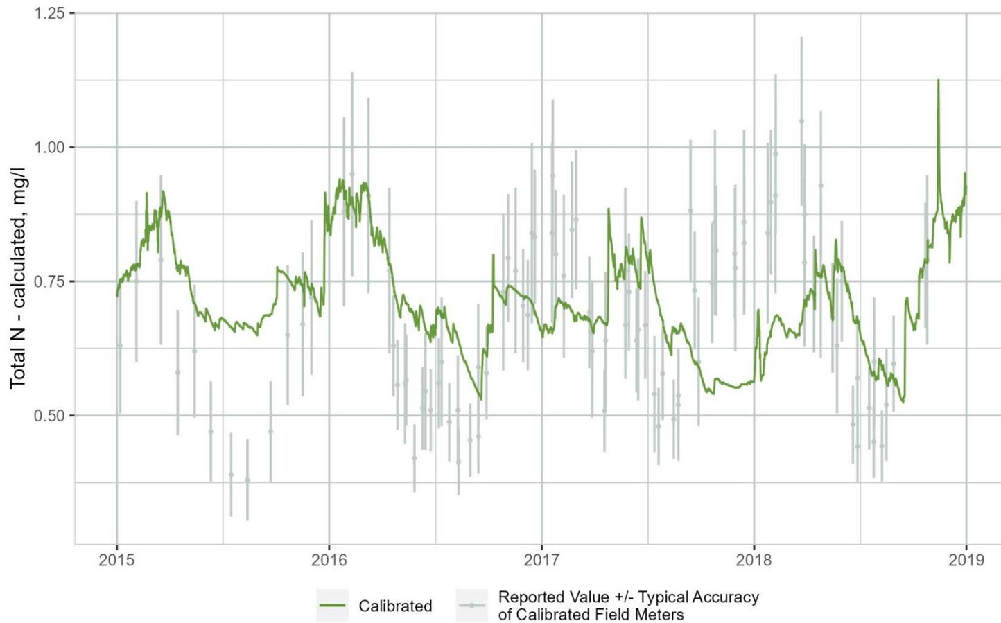
**Figure B-38. Time Series Comparison of WARMF Lake Simulated Total Nitrogen (TN) Concentrations to Observations Collected at the Downstream End of Segment 6**
