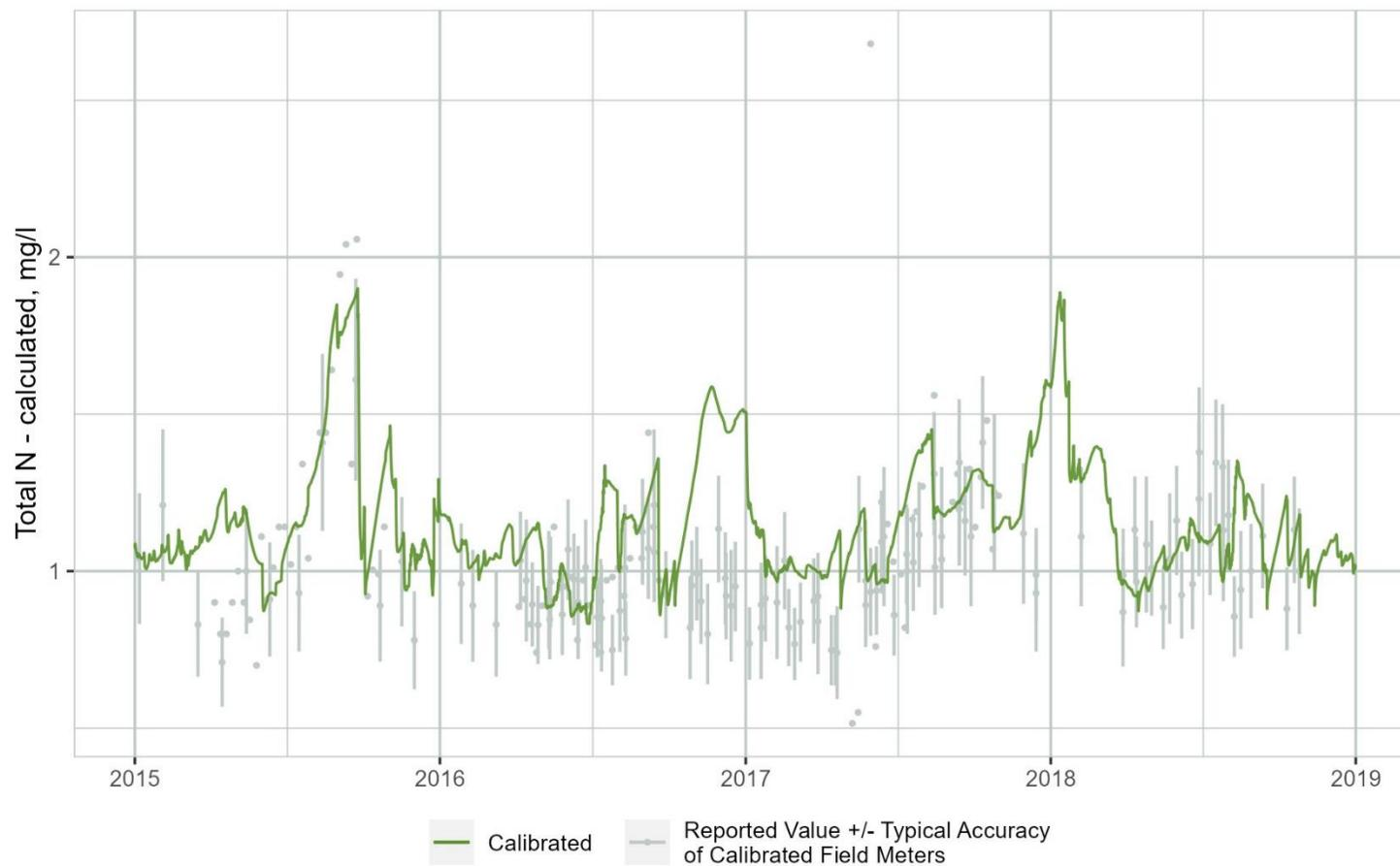
**Figure B-33. Time Series Comparison of WARMF Lake Simulated Total Nitrogen (TN) Concentrations to Observations Collected at the Downstream End of Segment 1**
