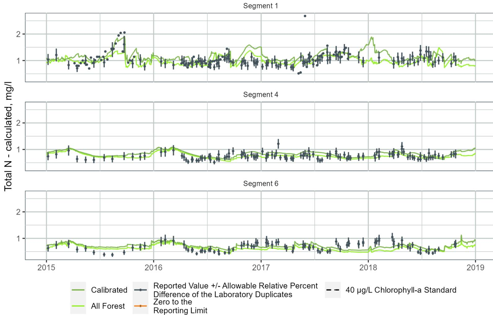
**Figure B-104. WARMF Lake Simulated Total Nitrogen Concentrations for the Calibrated Model Compared to the Instantaneous Land Conversion to All Forest with Elimination of Onsite and Centralized Wastewater Treatment Discharges and Nutrient Application to Land Surfaces (Atmospheric Deposition is not Altered from the Calibrated Model) in Segment 1 (upper lake near Interstate 85), Segment 4 (middle lake near Highway 50), and Segment 6 (lower lake near the dam)**
