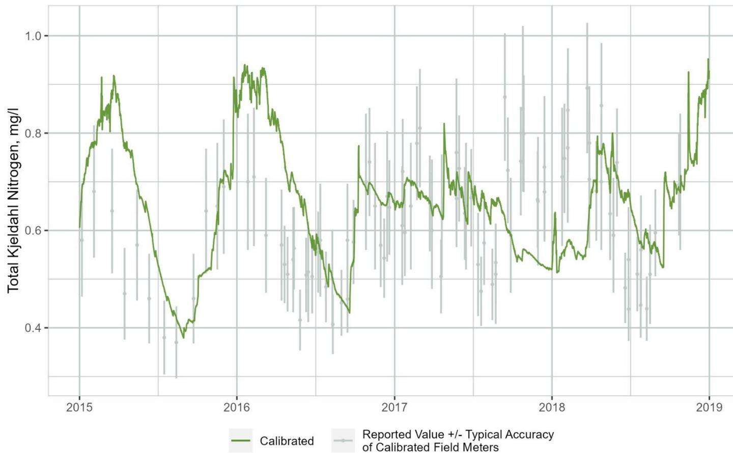
Figure B-32. Time Series Comparison of WARMF Lake Simulated Total Kjeldahl Nitrogen (TKN) Concentrations to Observations Collected at the Downstream End of Segment 6
