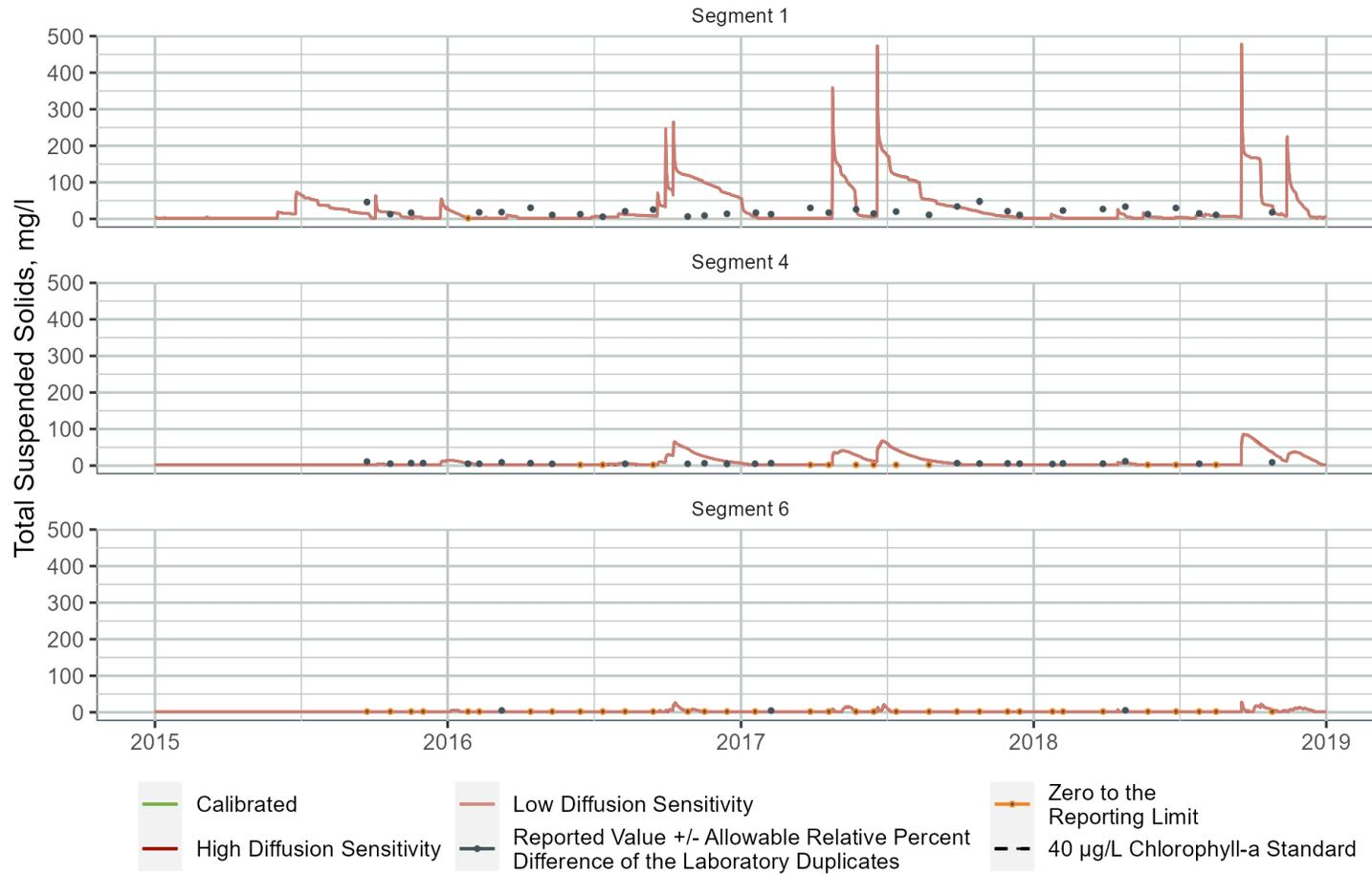
Figure B-86. TSS Sensitivity to Sediment Bed Diffusion Rate at Three WARMF Lake Segments
