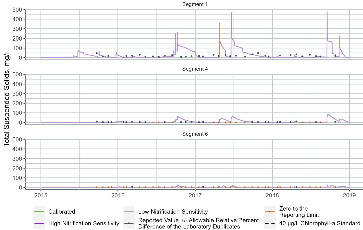
Figure B-94. TSS Sensitivity to Nitrification Rate at Three WARMF Lake Segments
