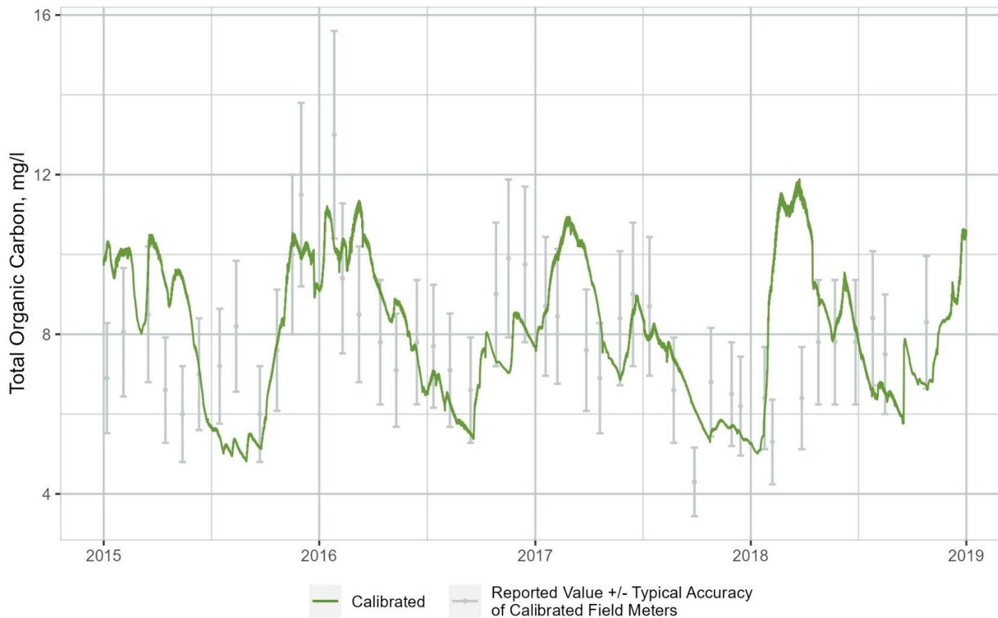
**Figure B-59. Time Series Comparison of WARMF Lake Simulated Total Organic Carbon (TOC) Concentrations to Observations Collected at the Downstream End of Segment 3**
