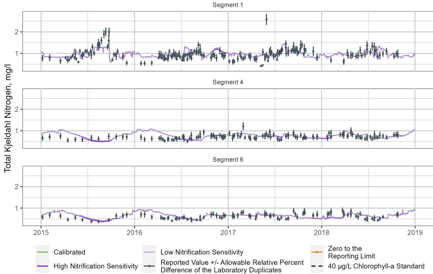
Figure B-90. TKN Sensitivity to Nitrification Rate at Three WARMF Lake Segments
