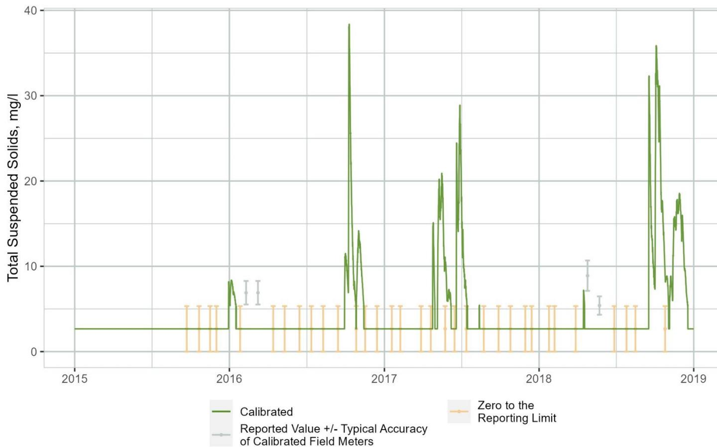
**Figure B-43. Time Series Comparison of WARMF Lake Simulated Total Suspended Sediment (TSS) Concentrations to Observations Collected at the Downstream End of Segment 5**
