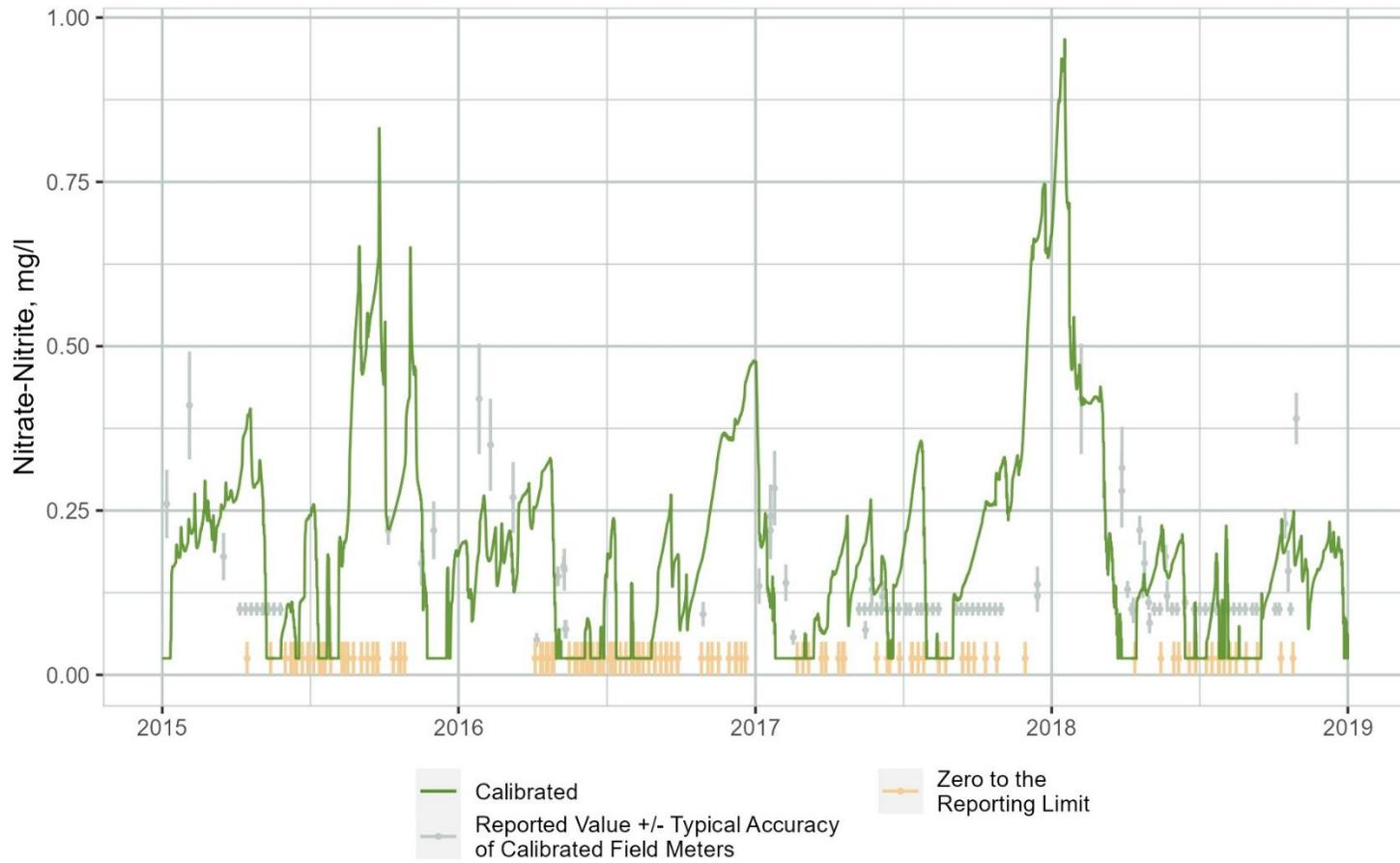
**Figure B-21. Time Series Comparison of WARMF Lake Simulated Nitrate plus Nitrite Concentrations to Observations Collected at the Downstream End of Segment 1**
