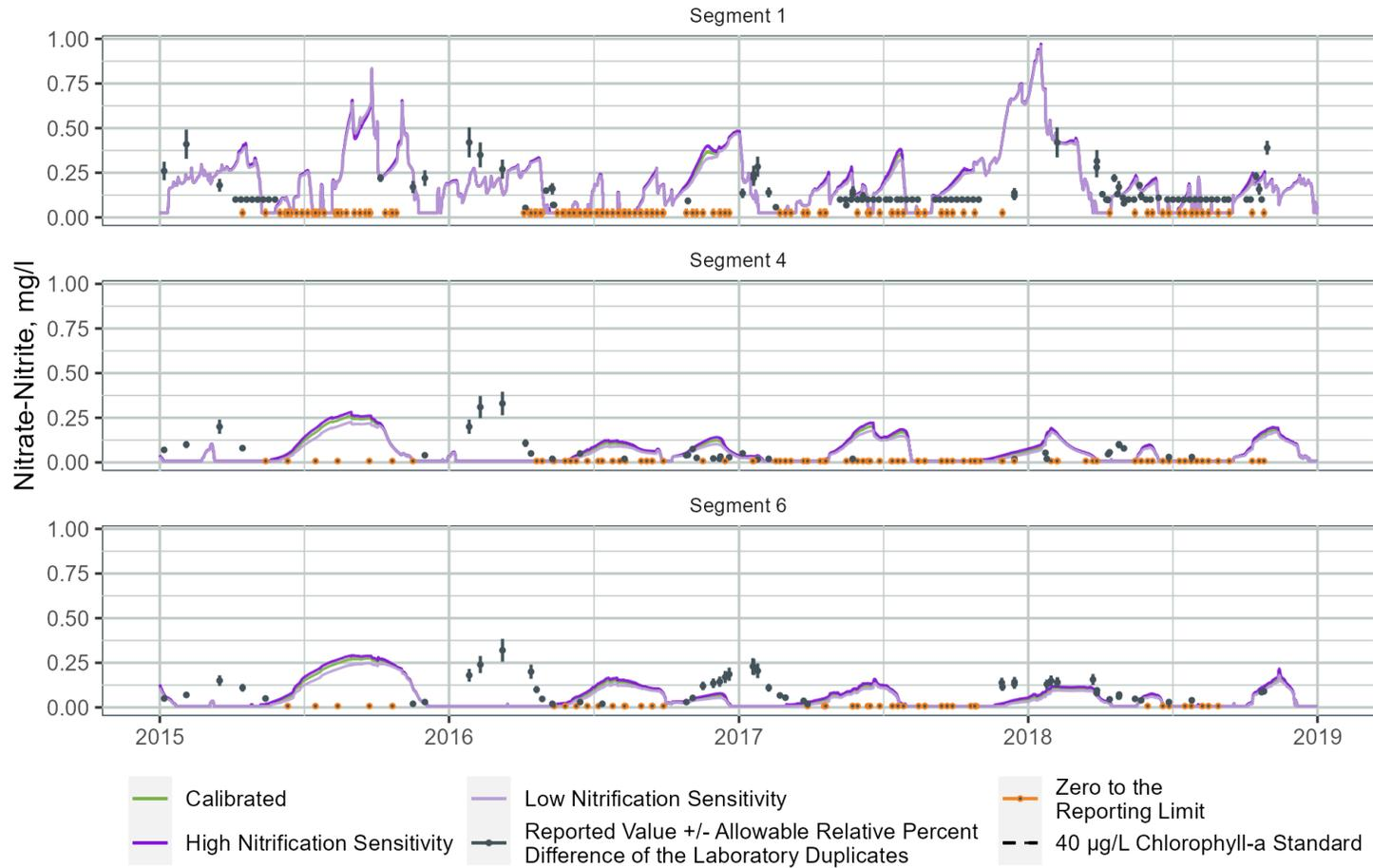
**Figure B-89. Nitrate plus Nitrite Sensitivity to Nitrification Rate at Three WARMF Lake Segments**
