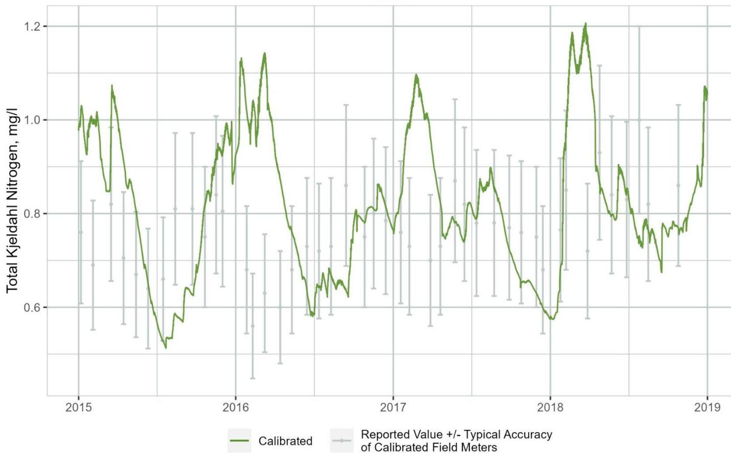
**Figure B-29. Time Series Comparison of WARMF Lake Simulated Total Kjeldahl Nitrogen (TKN) Concentrations to Observations Collected at the Downstream End of Segment 3**
