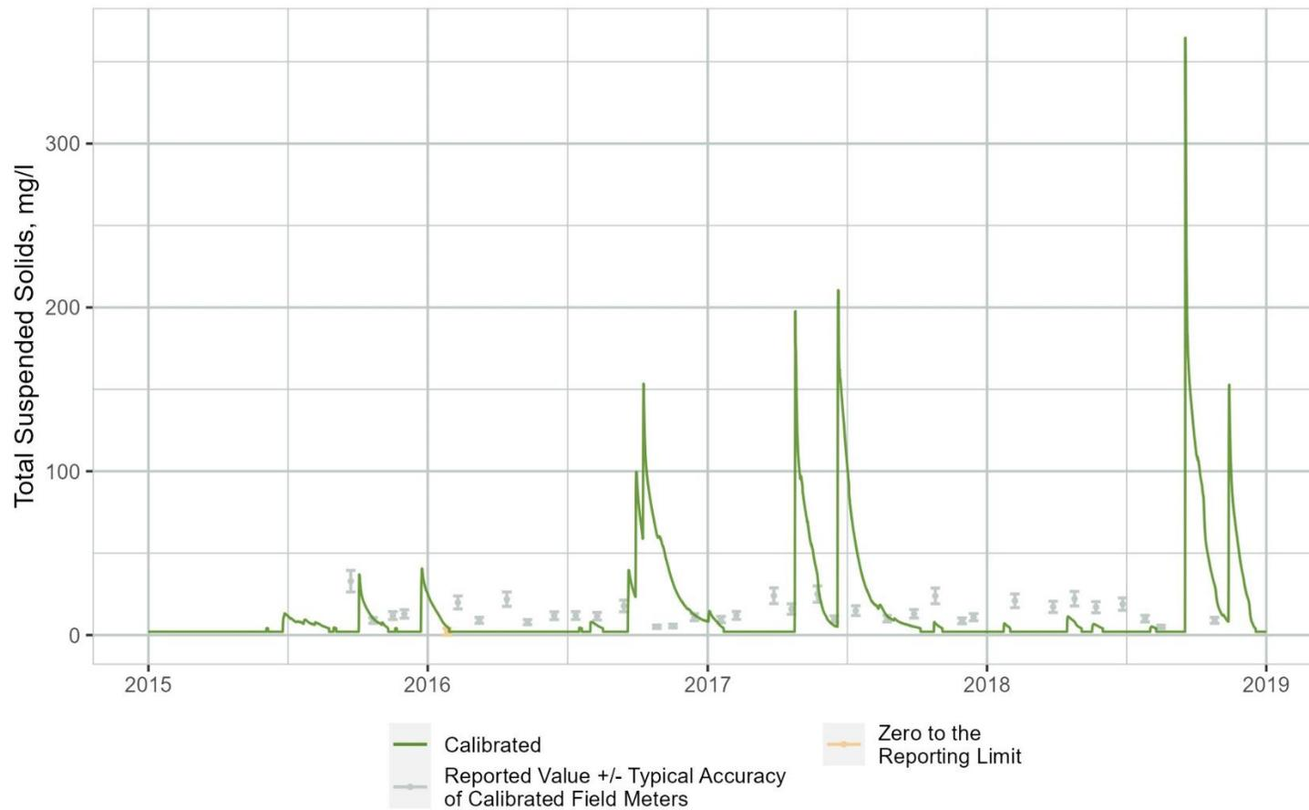
**Figure B-40. Time Series Comparison of WARMF Lake Simulated Total Suspended Sediment (TSS) Concentrations to Observations Collected at the Downstream End of Segment 2**
