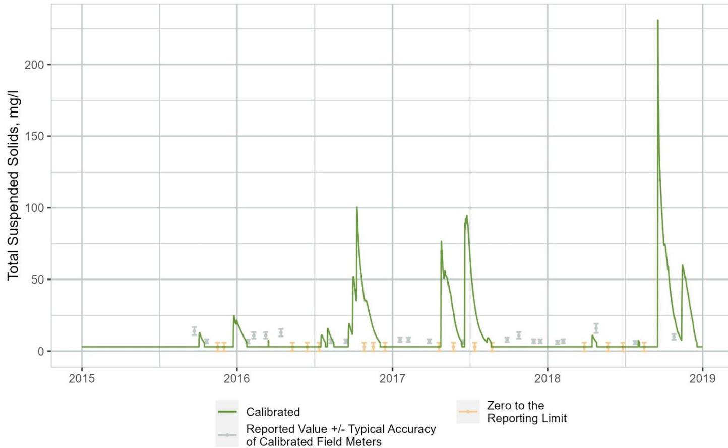
**Figure B-41. Time Series Comparison of WARMF Lake Simulated Total Suspended Sediment (TSS) Concentrations to Observations Collected at the Downstream End of Segment 3**
