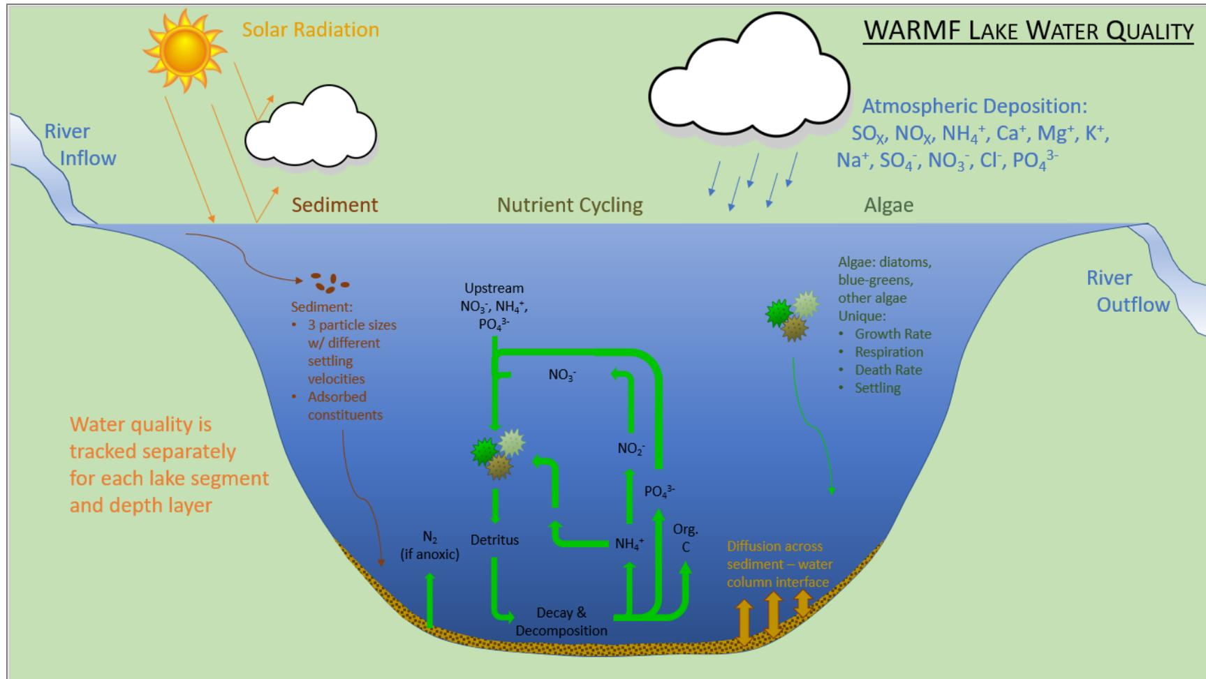
Figure B-3. Conceptual diagram of the WARMF Lake Water Quality Model
