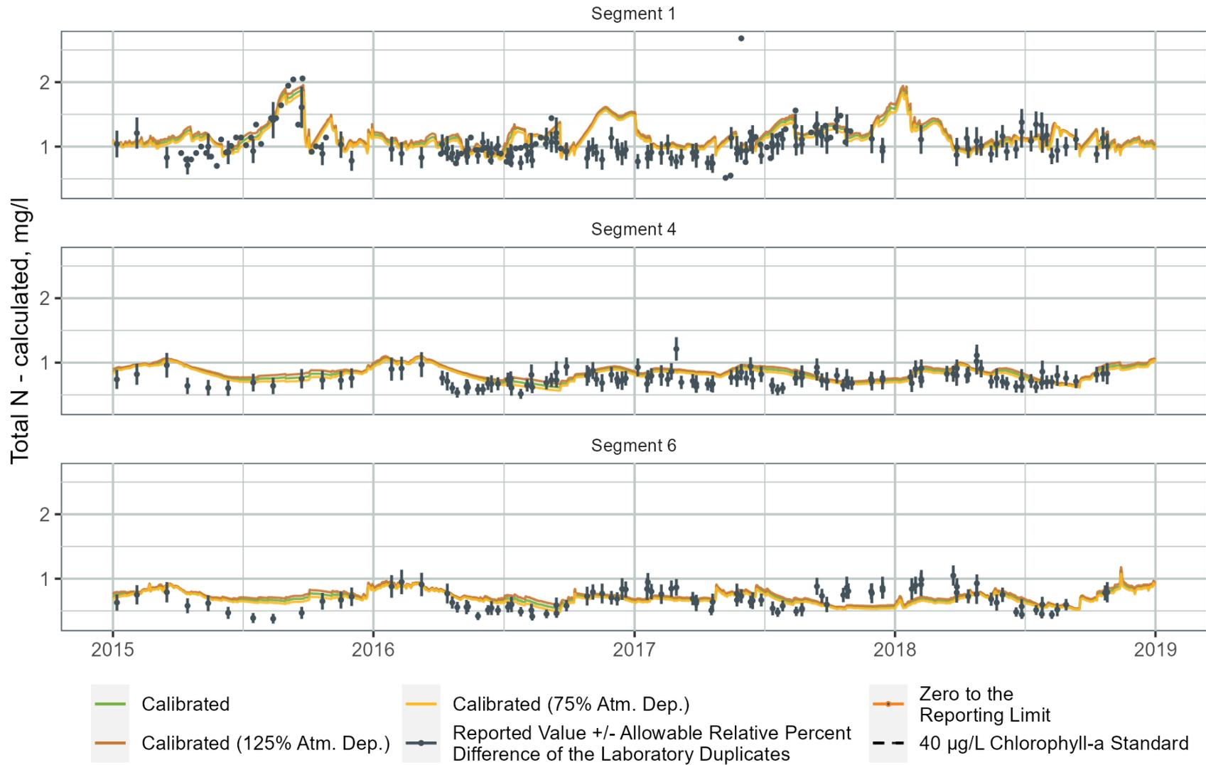
**Figure B-108. WARMF Lake Simulated Total Nitrogen Concentrations for the Calibrated Model Compared to 25 Percent Increase or Decrease in Atmospheric Deposition of Total Nitrogen, Total Phosphorus, and Total Organic Carbon in Segment 1 (upper lake near Interstate 85), Segment 4 (middle lake near Highway 50), and Segment 6 (lower lake near the dam)**
