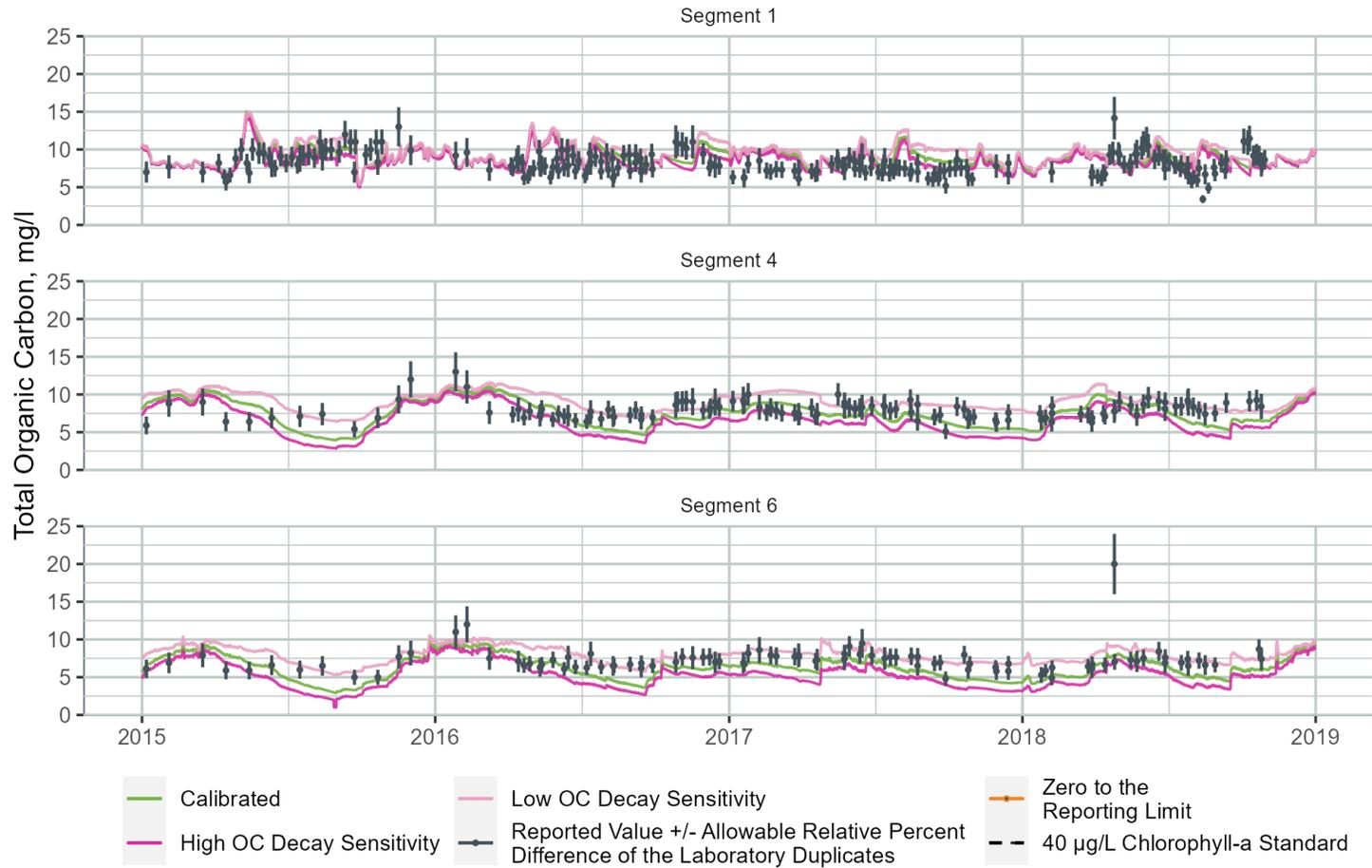
Figure B-100. TOC Sensitivity to Organic Matter Decay Rate at Three WARMF Lake Segments
