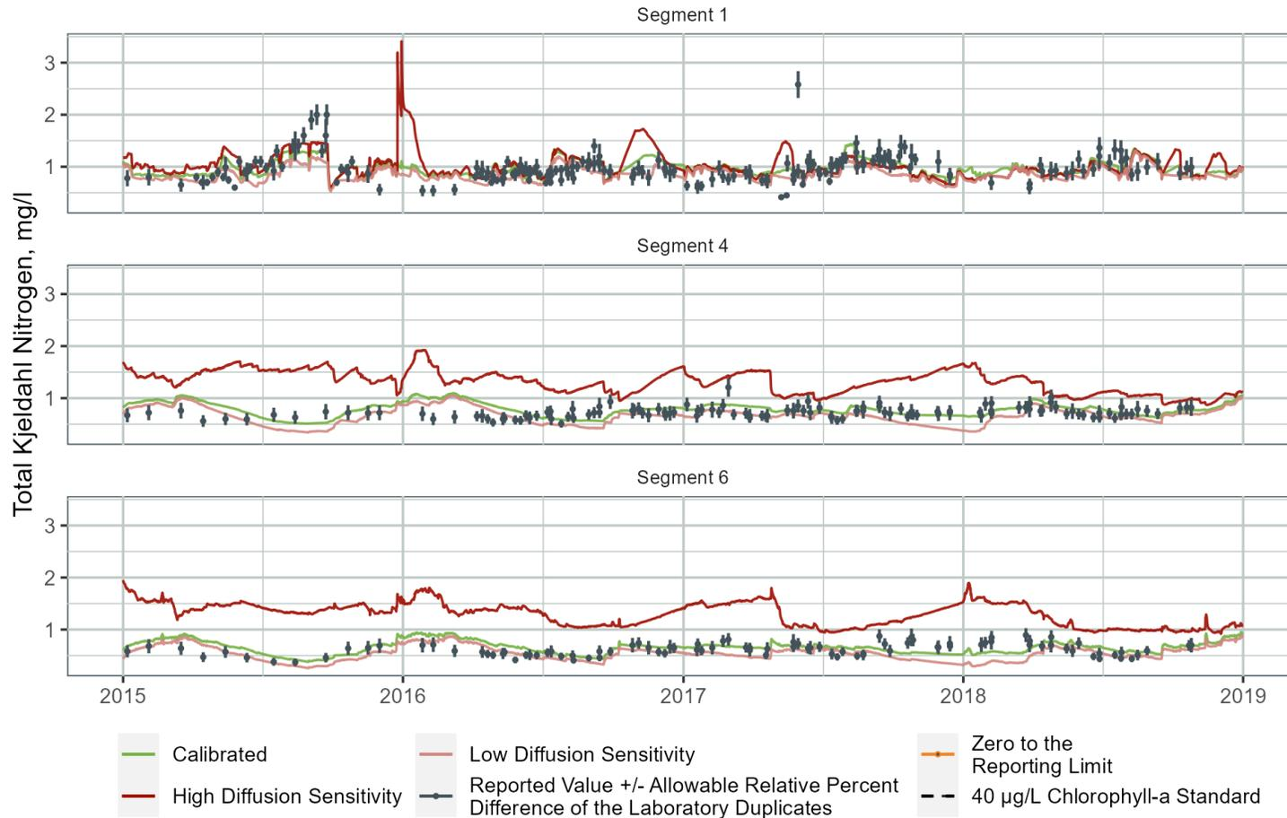
Figure B-82. TKN Sensitivity to Sediment Bed Diffusion Rate at Three WARMF Lake Segments
