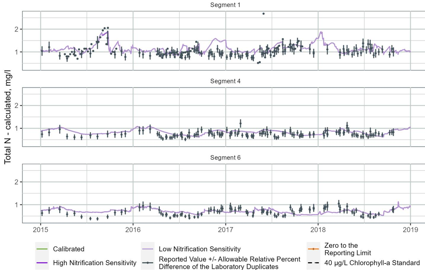
Figure B-91. TN Sensitivity to Nitrification Rate at Three WARMF Lake Segments
