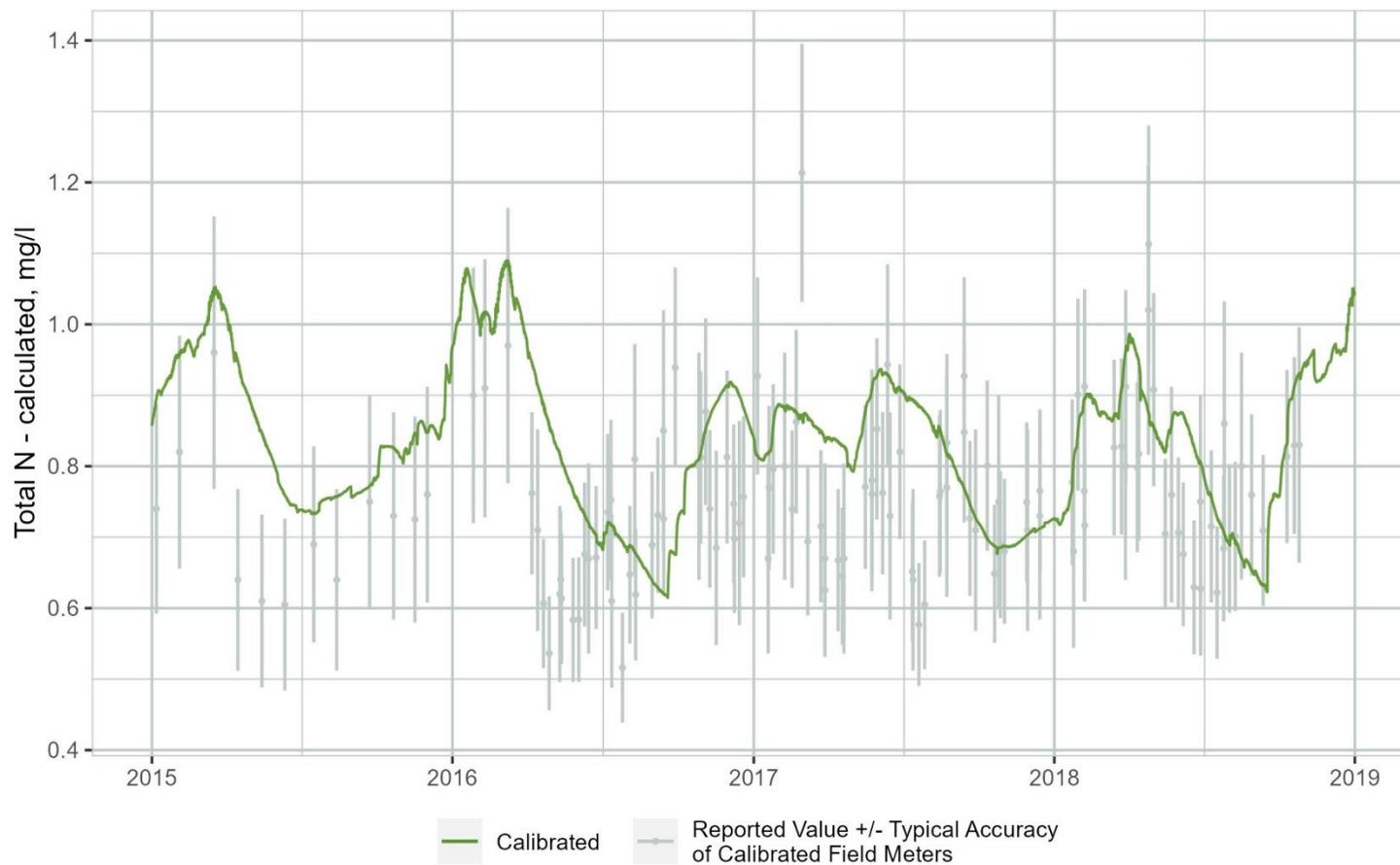
**Figure B-36. Time Series Comparison of WARMF Lake Simulated Total Nitrogen (TN) Concentrations to Observations Collected at the Downstream End of Segment 4**
