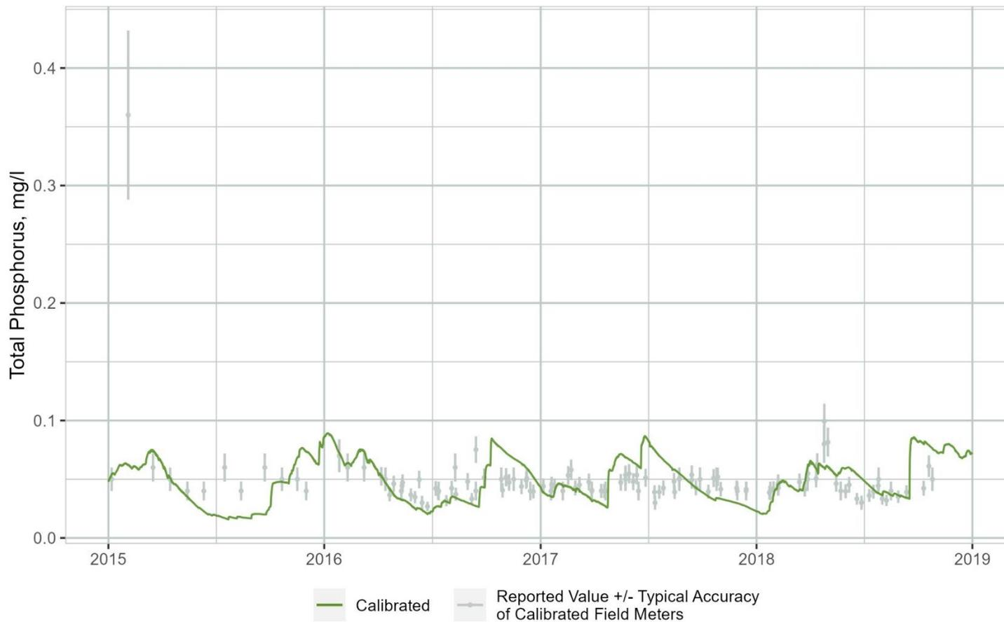
**Figure B-48. Time Series Comparison of WARMF Lake Simulated Total Phosphorus (TP) Concentrations to Observations Collected at the Downstream End of Segment 4**
