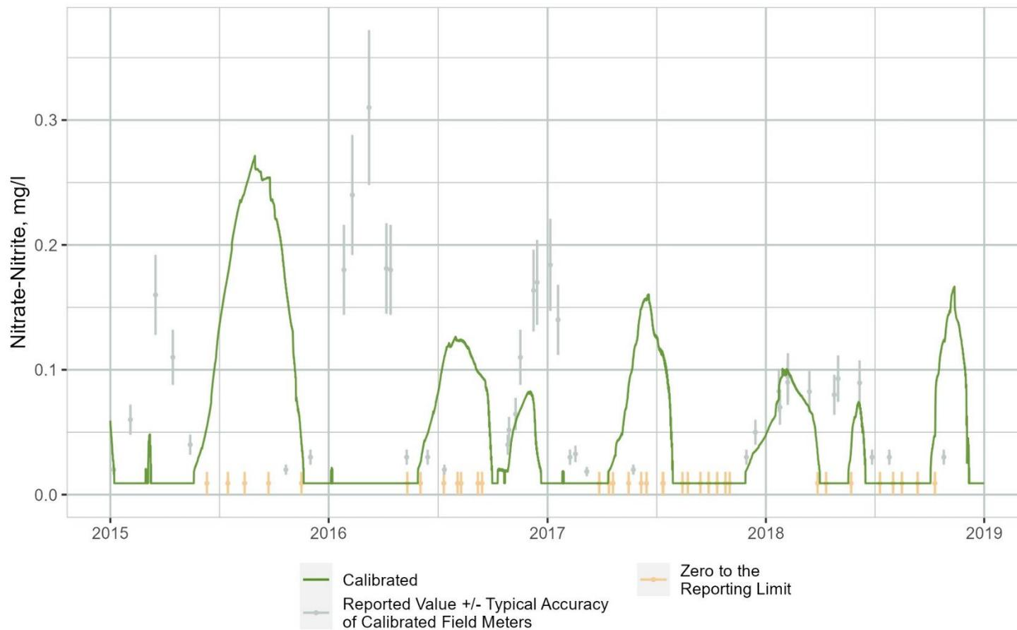
Figure B-25. Time Series Comparison of WARMF Lake Simulated Nitrate plus Nitrite Concentrations to Observations Collected at the Downstream End of Segment 5
