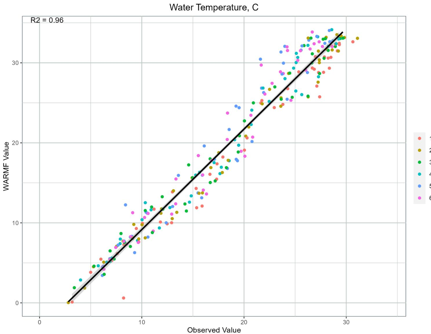
Figure B-63. Scatter Plot Comparing WARMF Lake Simulated Water Temperatures to Observations Collected in Falls Lake for Six Mainstem Segments
