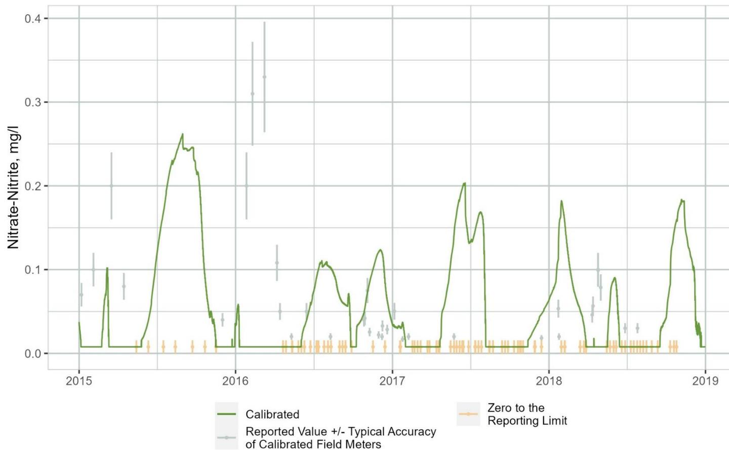
Figure B-24. Time Series Comparison of WARMF Lake Simulated Nitrate plus Nitrite Concentrations to Observations Collected at the Downstream End of Segment 4
