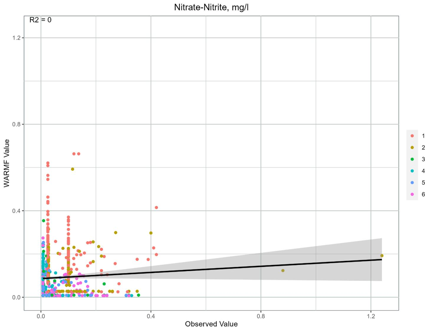
Figure B-65. Scatter Plot Comparing of WARMF Lake Simulated Nitrate plus Nitrite Concentrations to Observations Collected in Falls Lake for Six Mainstem Segments
