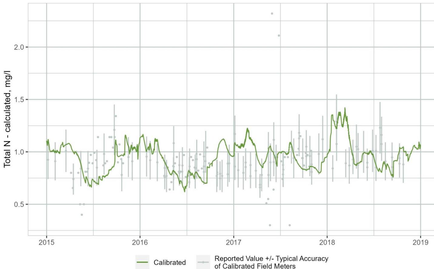
**Figure B-34. Time Series Comparison of WARMF Lake Simulated Total Nitrogen (TN) Concentrations to Observations Collected at the Downstream End of Segment 2**
