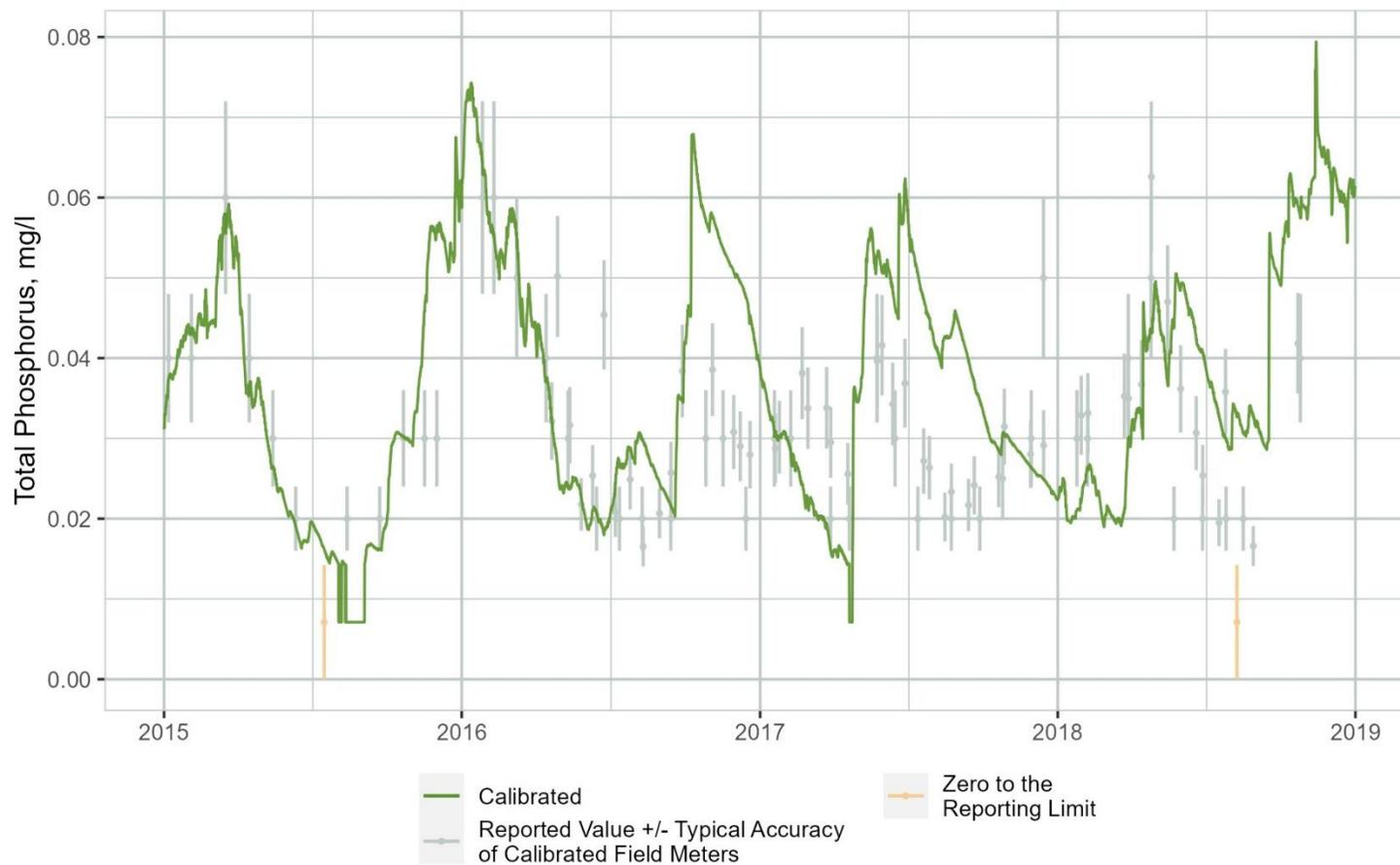
Figure B-50. Time Series Comparison of WARMF Lake Simulated Total Phosphorus (TP) Concentrations to Observations Collected at the Downstream End of Segment 6
