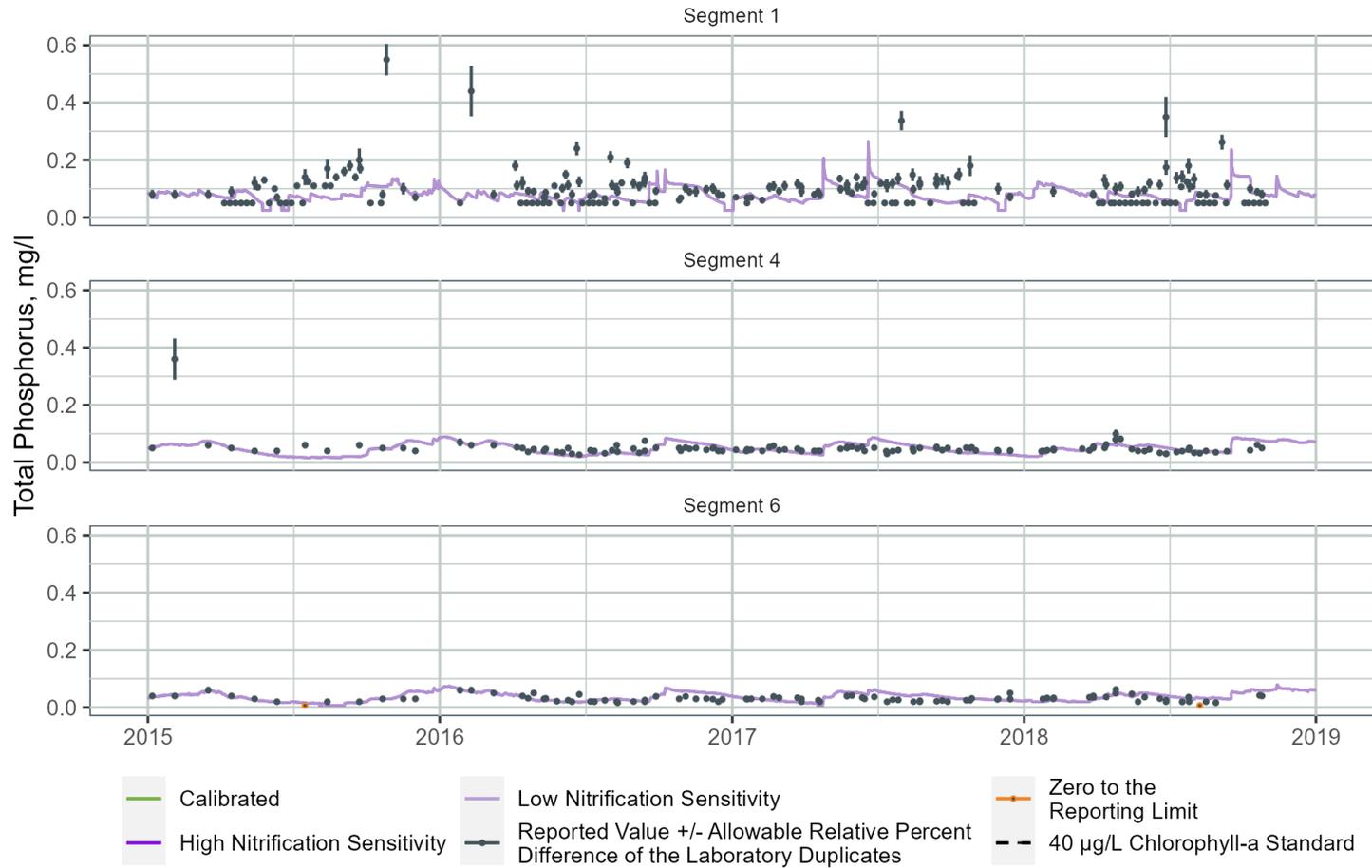
Figure B-93. TP Sensitivity to Nitrification Rate at Three WARMF Lake Segments
