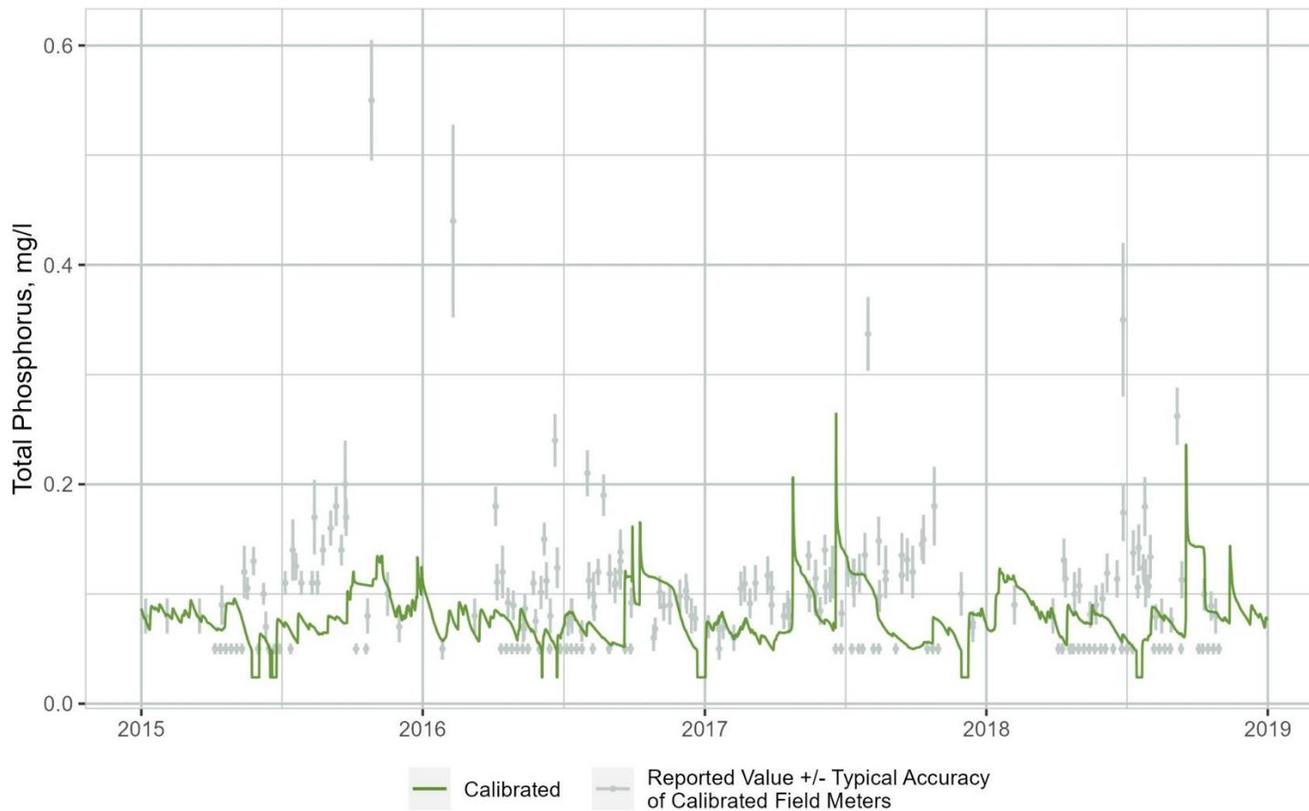
**Figure B-45. Time Series Comparison of WARMF Lake Simulated Total Phosphorus (TP) Concentrations to Observations Collected at the Downstream End of Segment 1**
