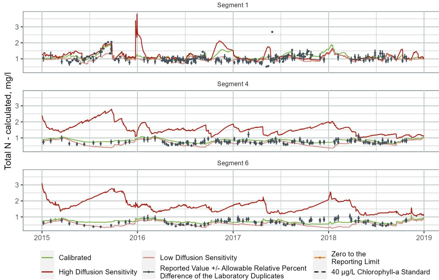
Figure B-83. TN Sensitivity to Sediment Bed Diffusion Rate at Three WARMF Lake Segments
