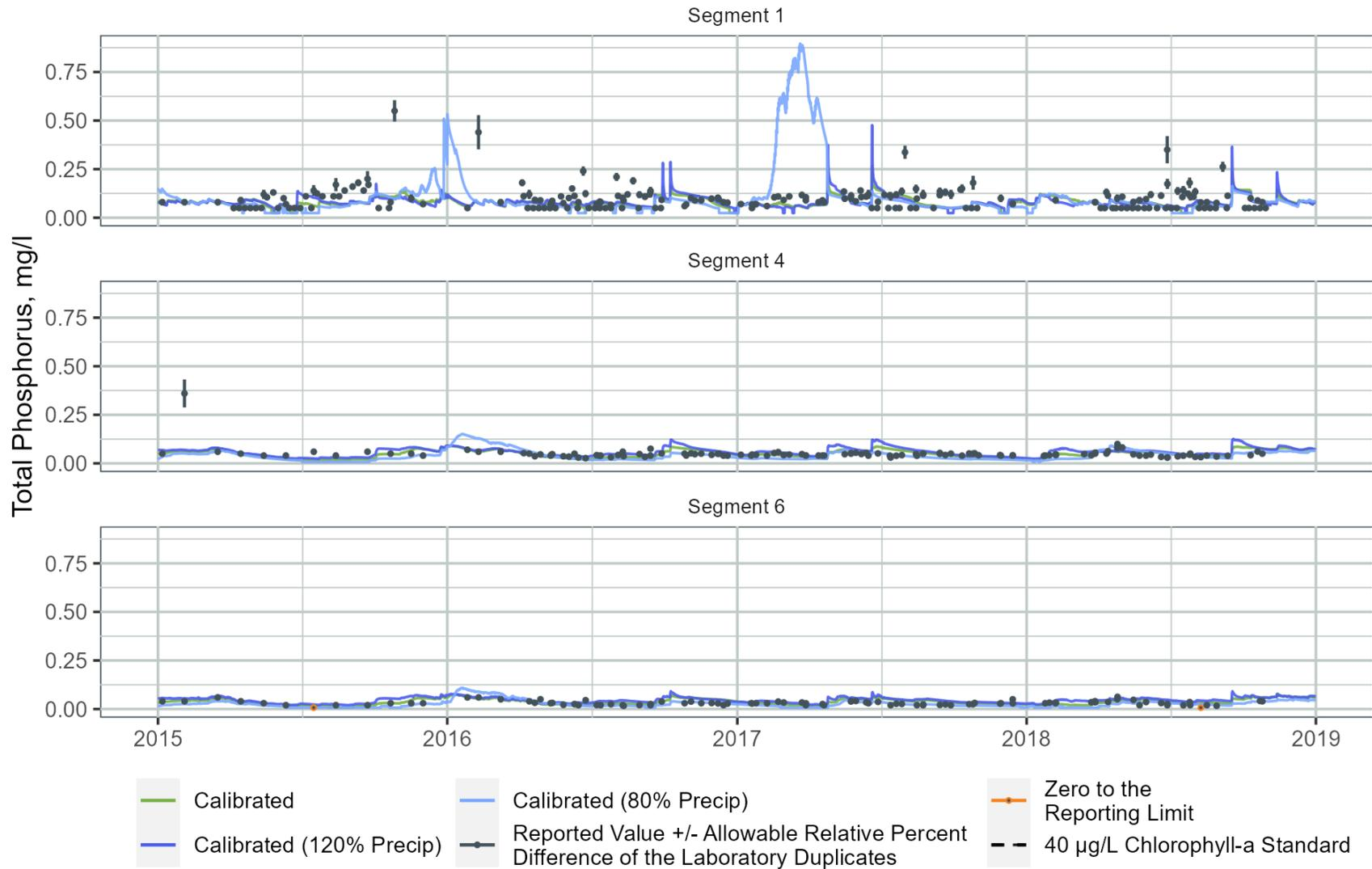
**Figure B-113. WARMF Lake Simulated Total Phosphorus Concentrations for the Calibrated Model Compared to 20 Percent Increase or Decrease in Rainfall Amount in Segment 1 (upper lake near Interstate 85), Segment 4 (middle lake near Highway 50), and Segment 6 (lower lake near the dam)**
