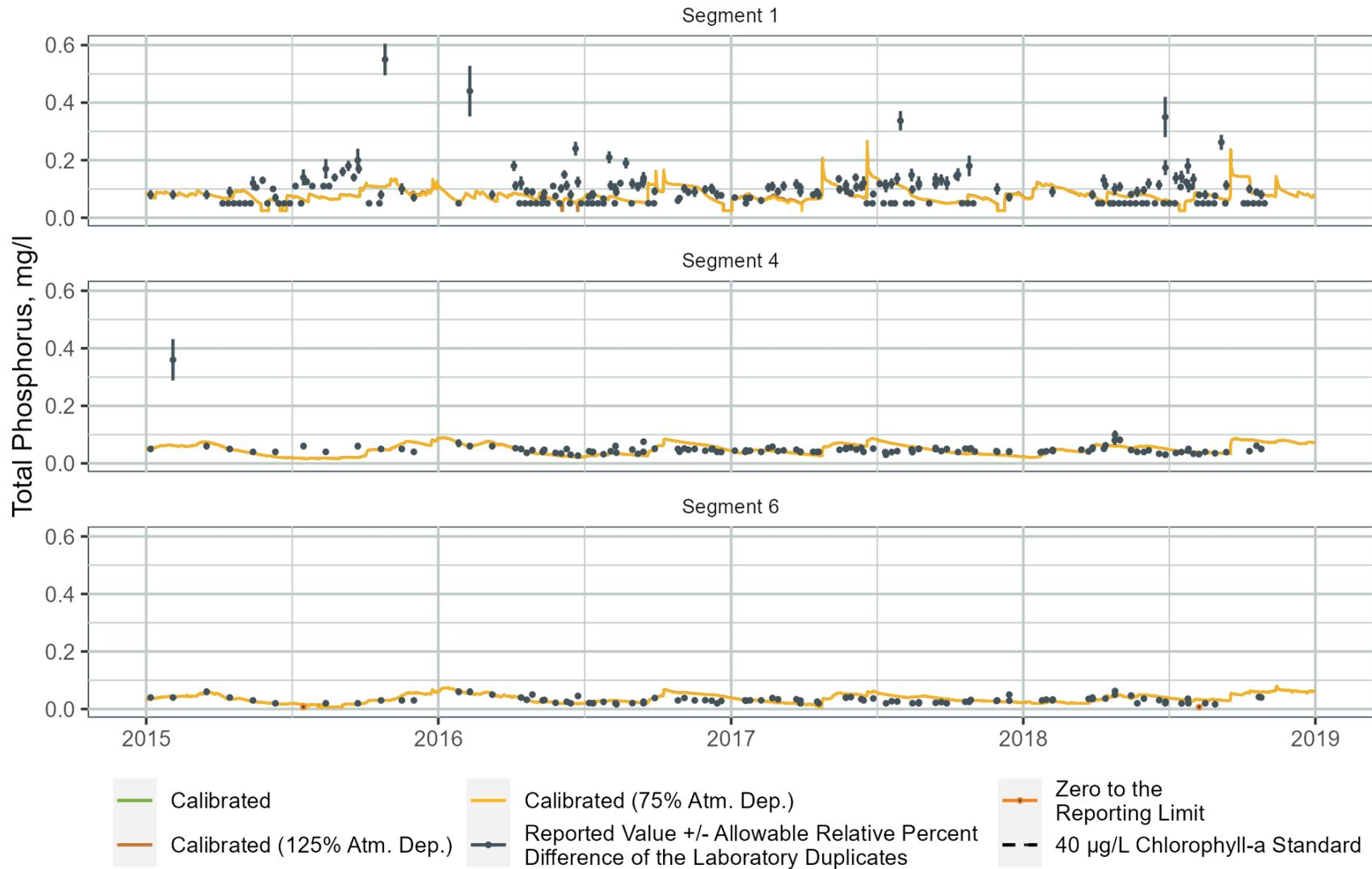
**Figure B-109. WARMF Lake Simulated Total Phosphorus Concentrations for the Calibrated Model Compared to 25 Percent Increase or Decrease in Atmospheric Deposition of Total Nitrogen, Total Phosphorus, and Total Organic Carbon in Segment 1 (upper lake near Interstate 85), Segment 4 (middle lake near Highway 50), and Segment 6 (lower lake near the dam)**
