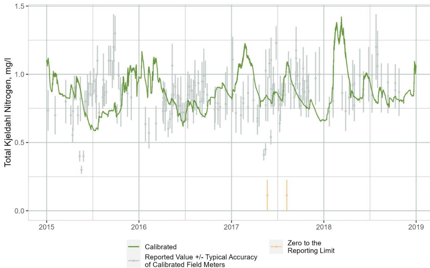
**Figure B-28. Time Series Comparison of WARMF Lake Simulated Total Kjeldahl Nitrogen (TKN) Concentrations to Observations Collected at the Downstream End of Segment 2**
