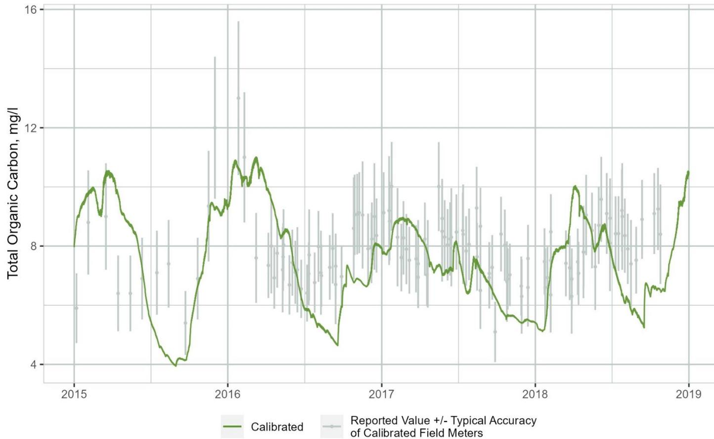
**Figure B-60. Time Series Comparison of WARMF Lake Simulated Total Organic Carbon (TOC) Concentrations to Observations Collected at the Downstream End of Segment 4**
