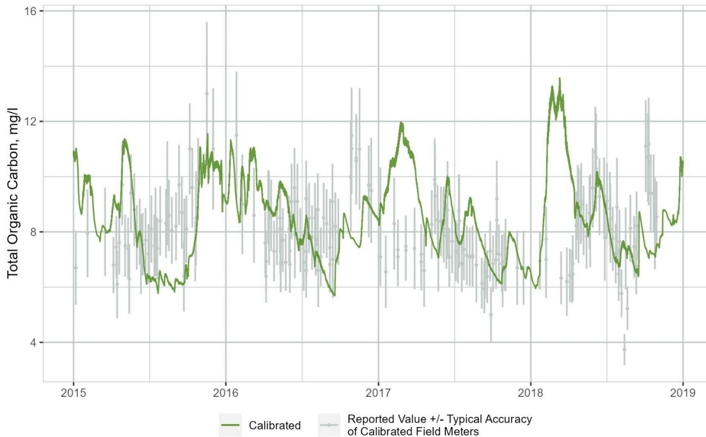
**Figure B-58. Time Series Comparison of WARMF Lake Simulated Total Organic Carbon (TOC) Concentrations to Observations Collected at the Downstream End of Segment 2**
