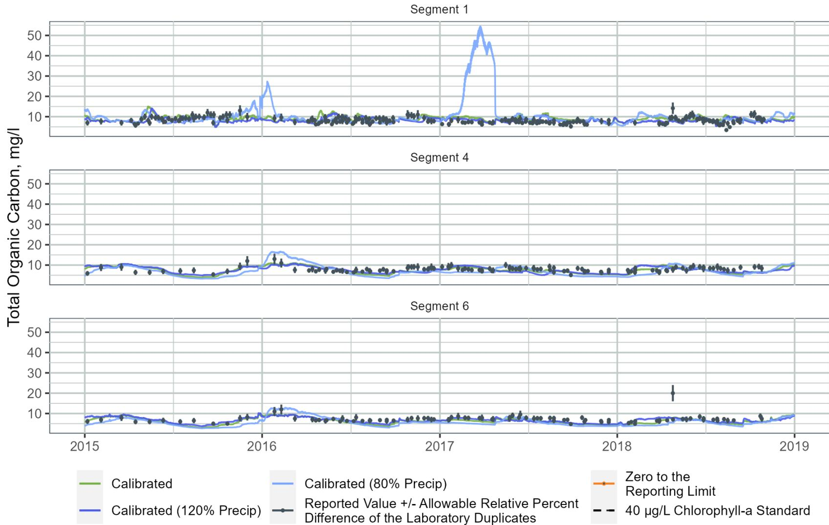
**Figure B-115. WARMF Lake Simulated Total Organic Carbon Concentrations for the Calibrated Model Compared to 20 Percent Increase or Decrease in Rainfall Amount in Segment 1 (upper lake near Interstate 85), Segment 4 (middle lake near Highway 50), and Segment 6 (lower lake near the dam)**
