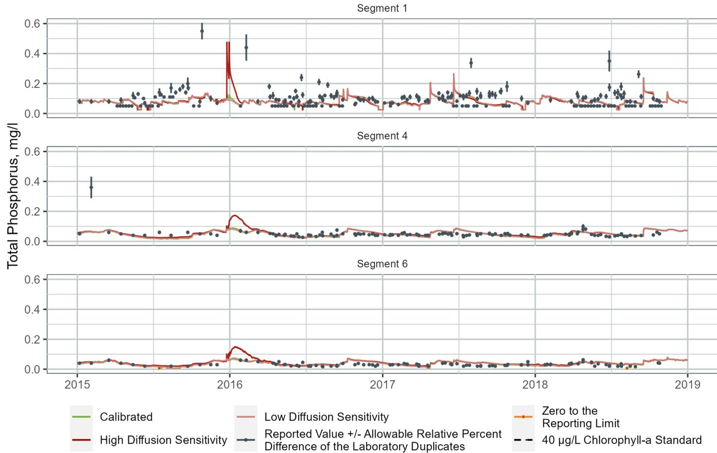
Figure B-85. TP Sensitivity to Sediment Bed Diffusion Rate at Three WARMF Lake Segments
