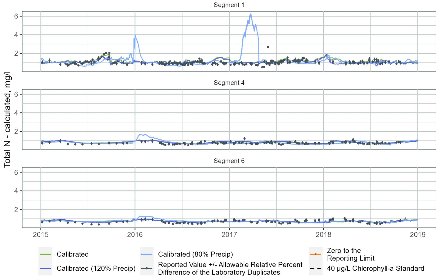
Figure B-112. WARMF Lake Simulated Total Nitrogen Concentrations for the Calibrated Model Compared to 20 Percent Increase or Decrease in Rainfall Amount in Segment 1 (upper lake near Interstate 85), Segment 4 (middle lake near Highway 50), and Segment 6 (lower lake near the dam)
