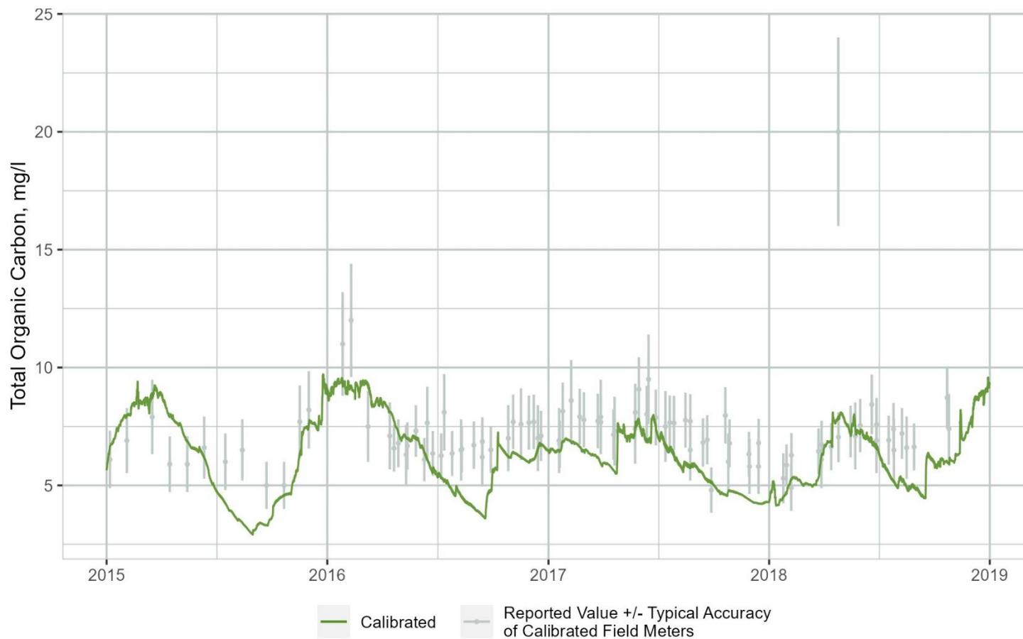
Figure B-62. Time Series Comparison of WARMF Lake Simulated Total Organic Carbon (TOC) Concentrations to Observations Collected at the Downstream End of Segment 6
