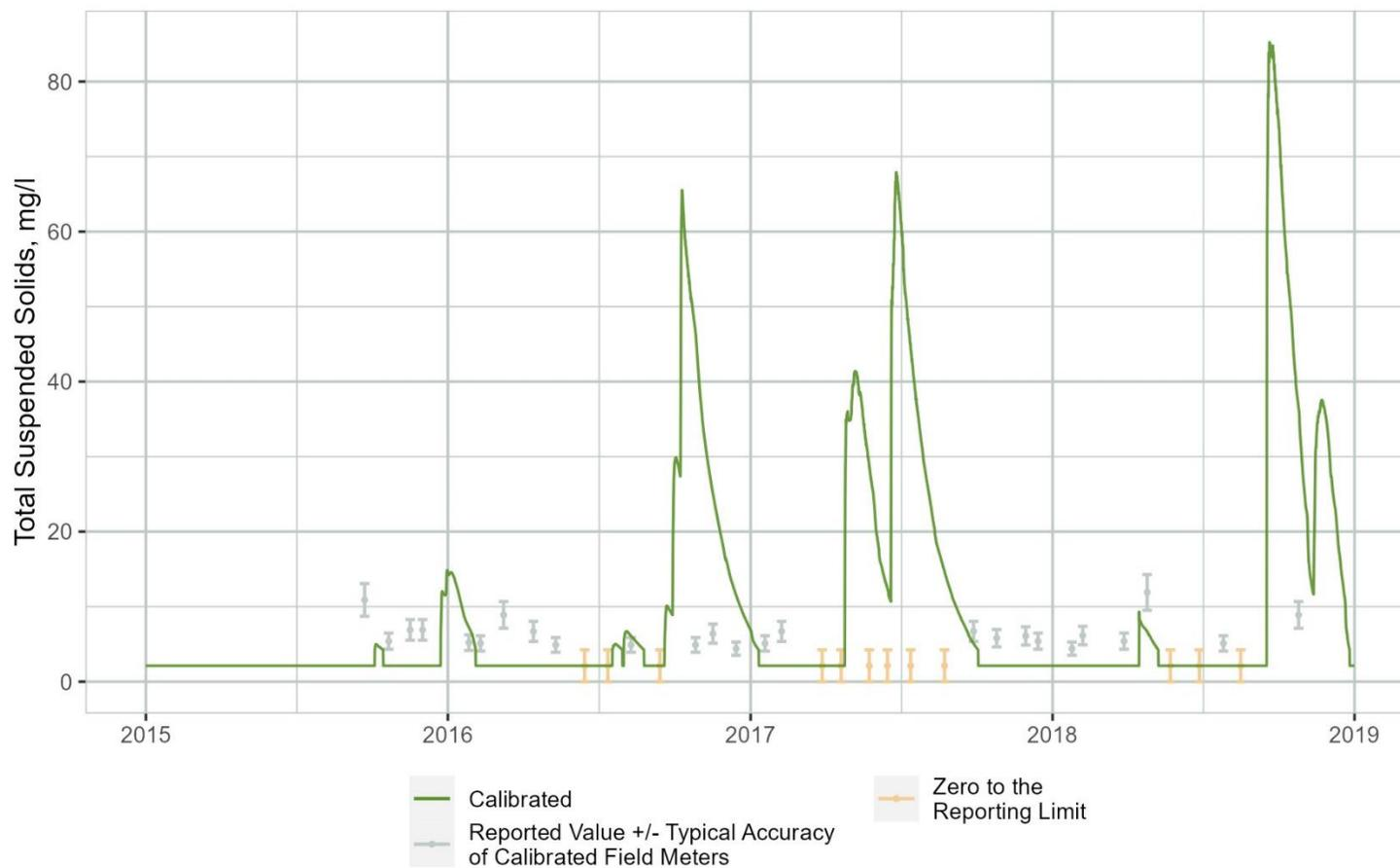
**Figure B-42. Time Series Comparison of WARMF Lake Simulated Total Suspended Sediment (TSS) Concentrations to Observations Collected at the Downstream End of Segment 4**
