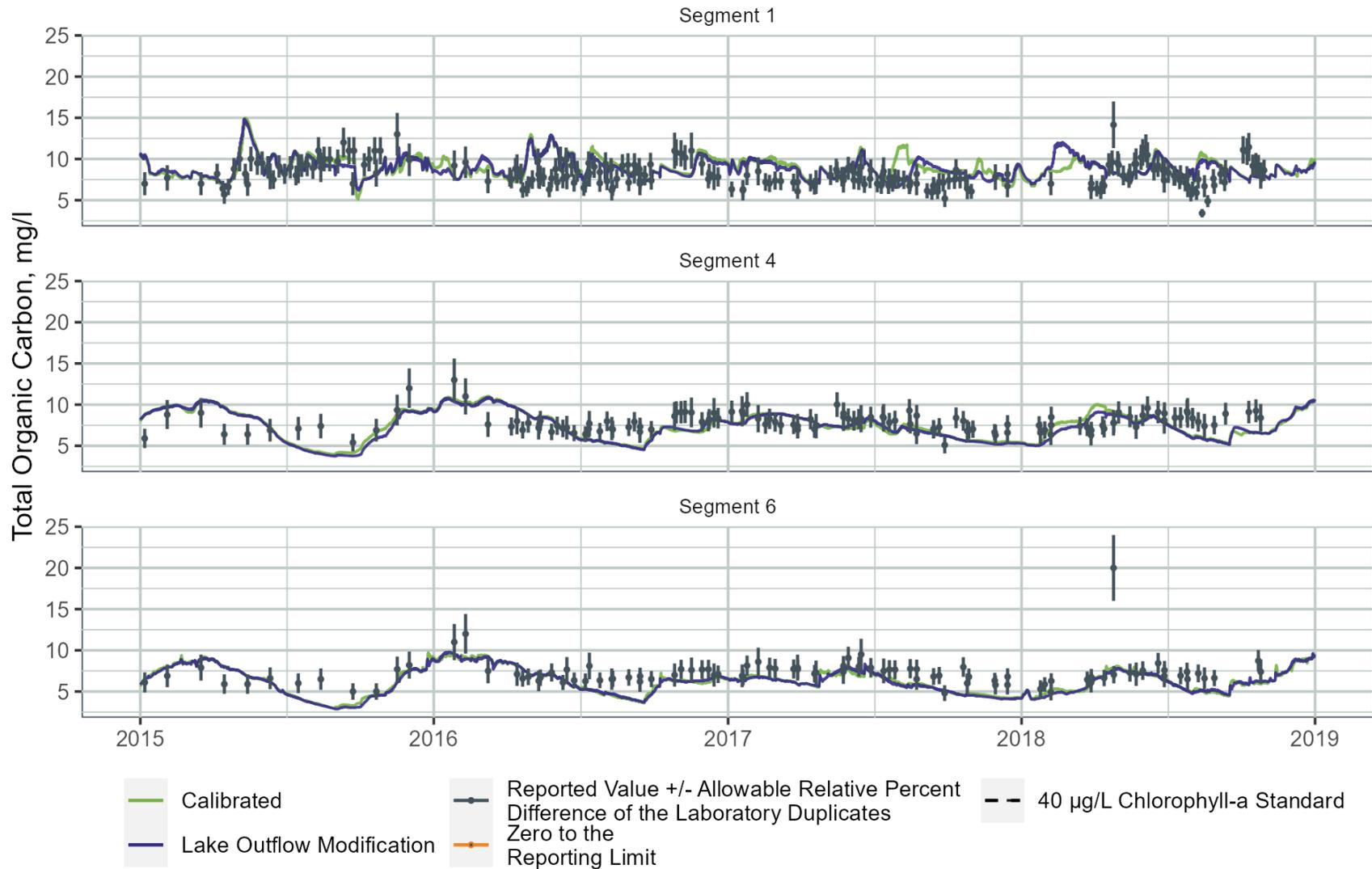
**Figure B-119. WARMF Lake Simulated Total Organic Carbon Concentrations for the Calibrated Model Compared to the Dam Release Scenario with the Spillway Elevation Set to Normal Pool in Segment 1 (upper lake near Interstate 85), Segment 4 (middle lake near Highway 50), and Segment 6 (lower lake near the dam)**
