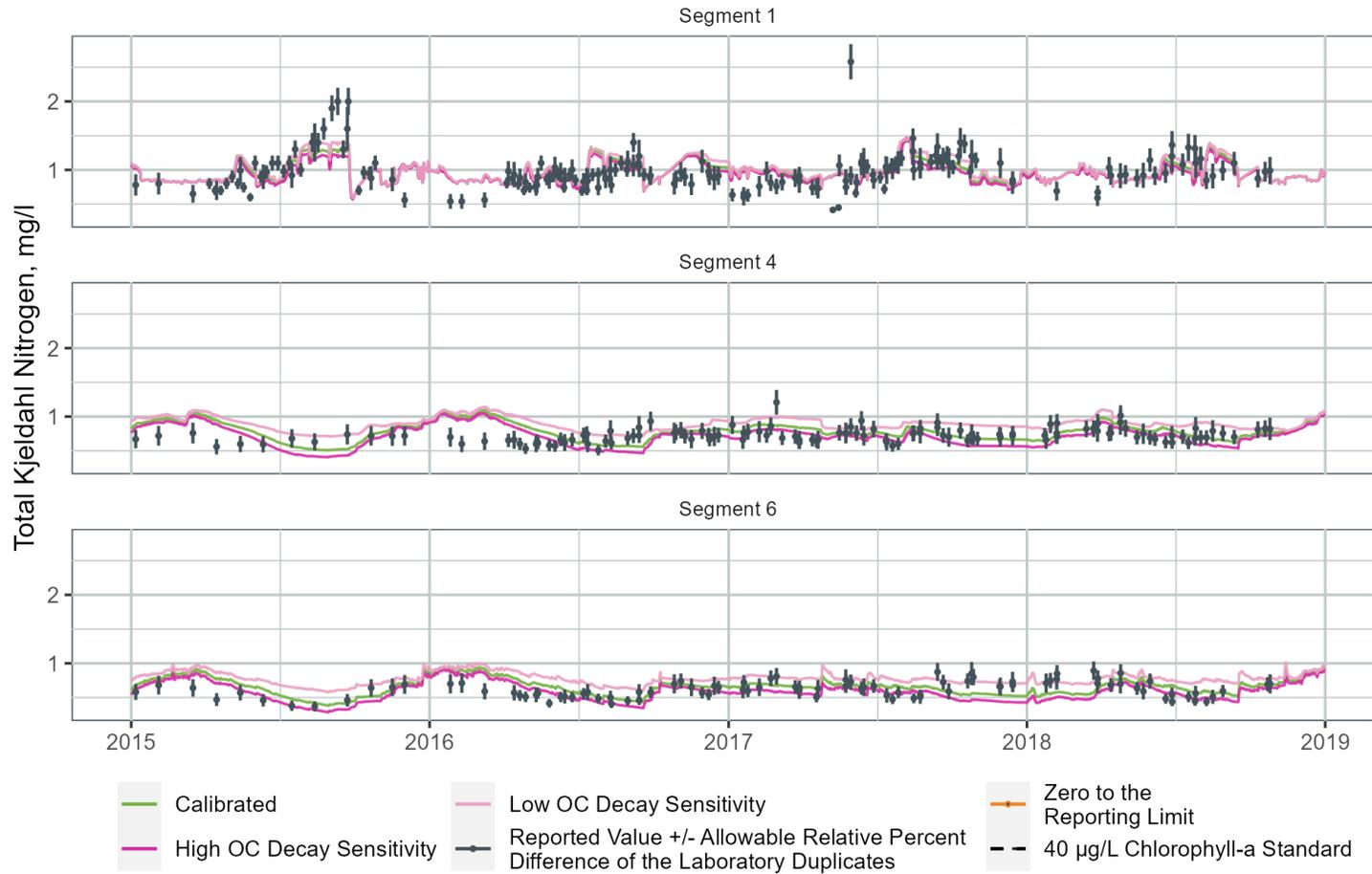
Figure B-98. TKN Sensitivity to Organic Matter Decay Rate at Three WARMF Lake Segments
