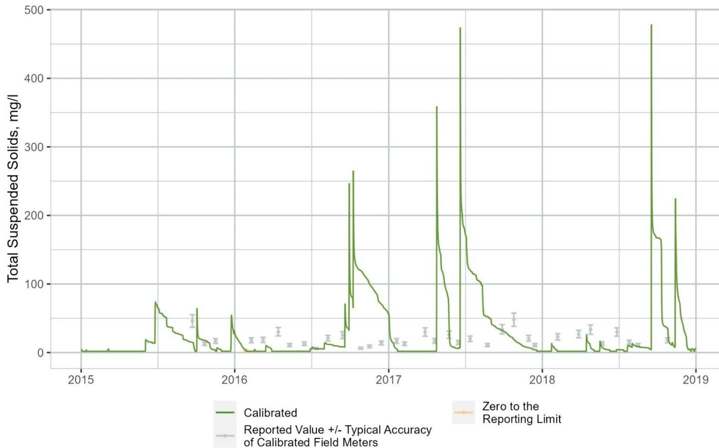
**Figure B-39. Time Series Comparison of WARMF Lake Simulated Total Suspended Sediment (TSS) Concentrations to Observations Collected at the Downstream End of Segment 1**
