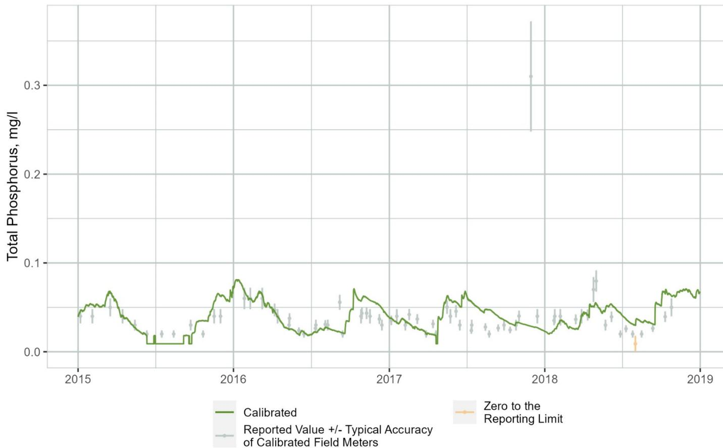
Figure B-49. Time Series Comparison of WARMF Lake Simulated Total Phosphorus (TP) Concentrations to Observations Collected at the Downstream End of Segment 5
