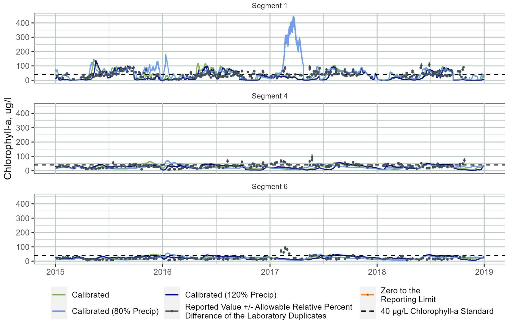
**Figure B-114. WARMF Lake Simulated Chlorophyll-a Concentrations for the Calibrated Model Compared to 20 Percent Increase or Decrease in Rainfall Amount in Segment 1 (upper lake near Interstate 85), Segment 4 (middle lake near Highway 50), and Segment 6 (lower lake near the dam)**
