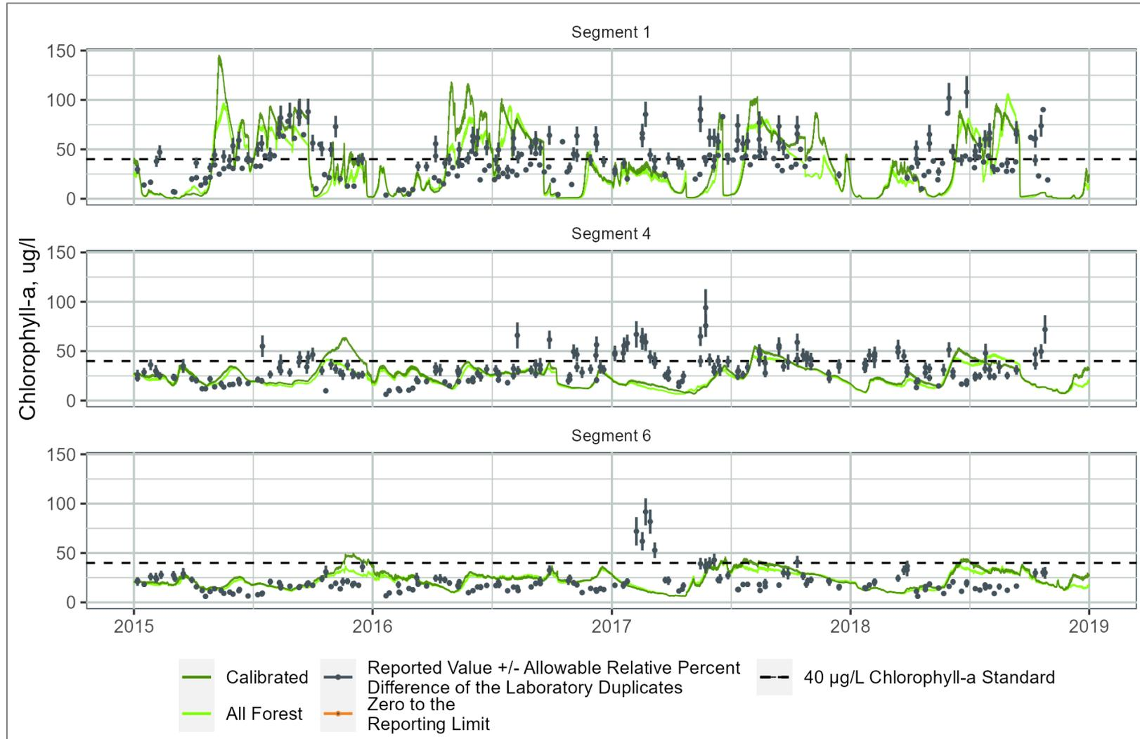
**Figure B-106. WARMF Lake Simulated Chlorophyll-a Concentrations for the Calibrated Model Compared to the Instantaneous Land Conversion to All Forest with Elimination of Onsite and Centralized Wastewater Treatment Discharges and Nutrient Application to Land Surfaces (Atmospheric Deposition is not Altered from the Calibrated Model) in Segment 1 (upper lake near Interstate 85), Segment 4 (middle lake near Highway 50), and Segment 6 (lower lake near the dam)**
