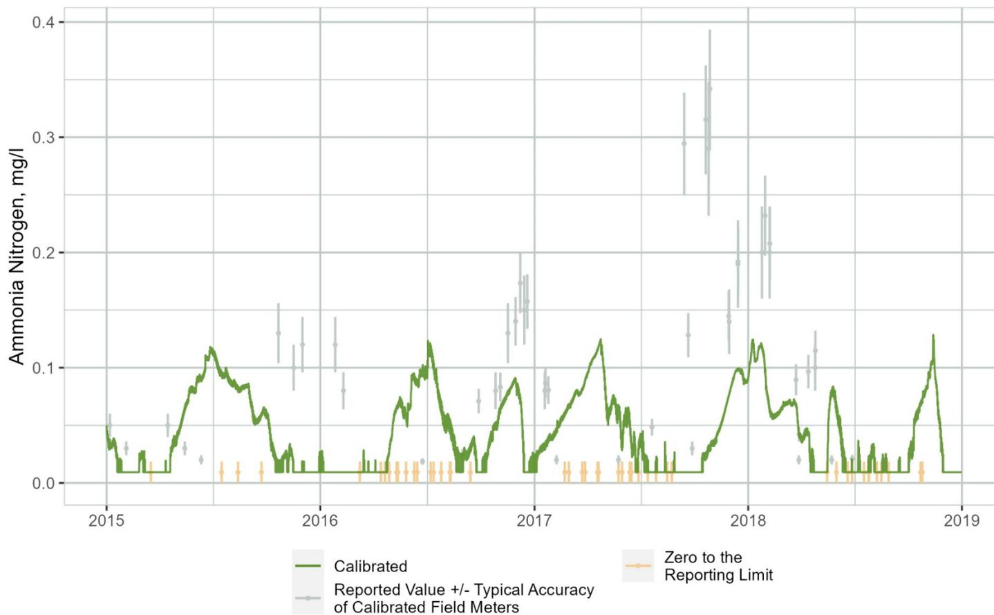
**Figure B-20. Time Series Comparison of WARMF Lake Simulated Ammonia Concentrations to Observations Collected at the Downstream End of Segment 6**
