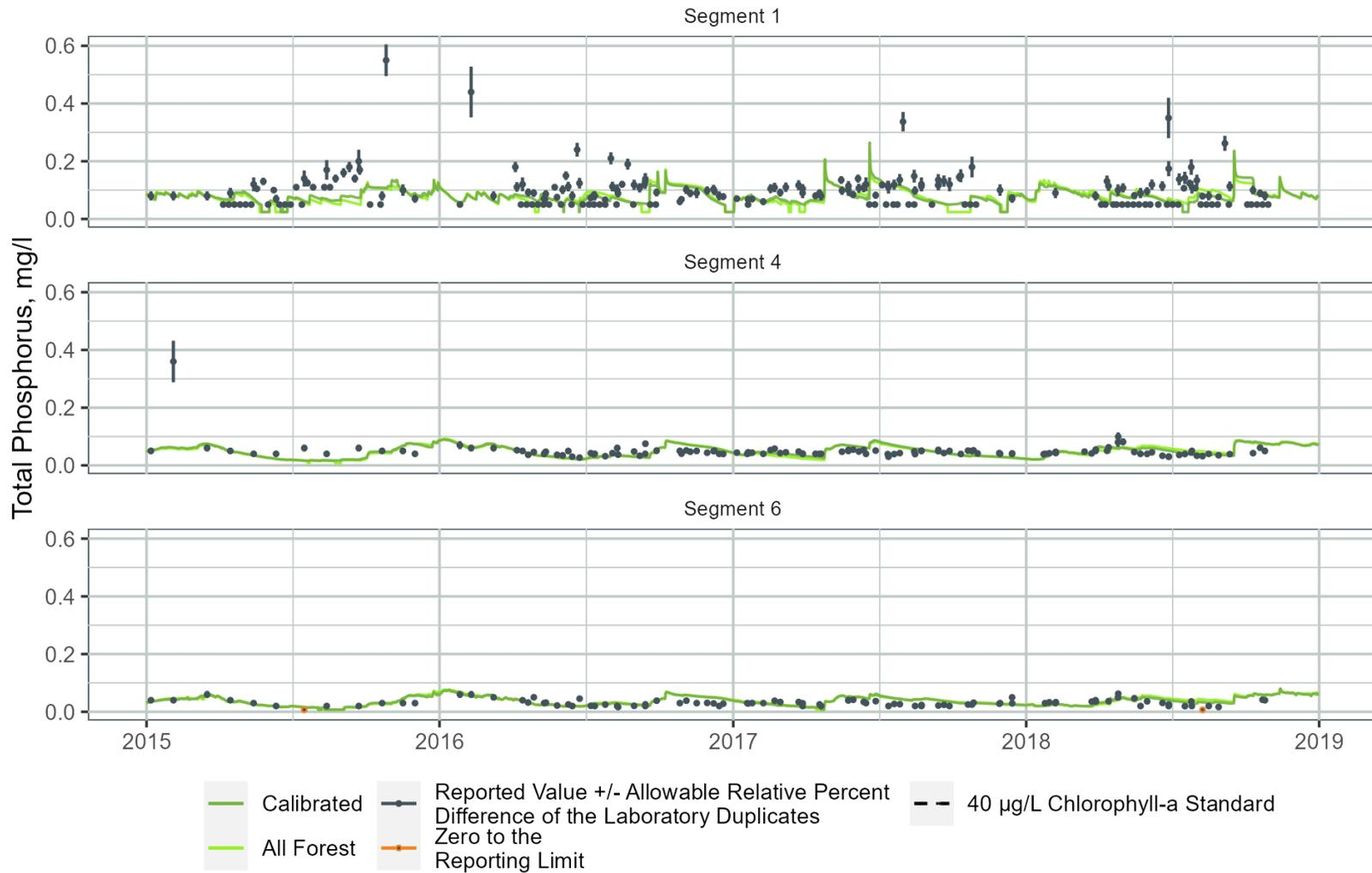
**Figure B-105. WARMF Lake Simulated Total Phosphorus Concentrations for the Calibrated Model Compared to the Instantaneous Land Conversion to All Forest with Elimination of Onsite and Centralized Wastewater Treatment Discharges and Nutrient Application to Land Surfaces (Atmospheric Deposition is not Altered from the Calibrated Model) in Segment 1 (upper lake near Interstate 85), Segment 4 (middle lake near Highway 50), and Segment 6 (lower lake near the dam)**
