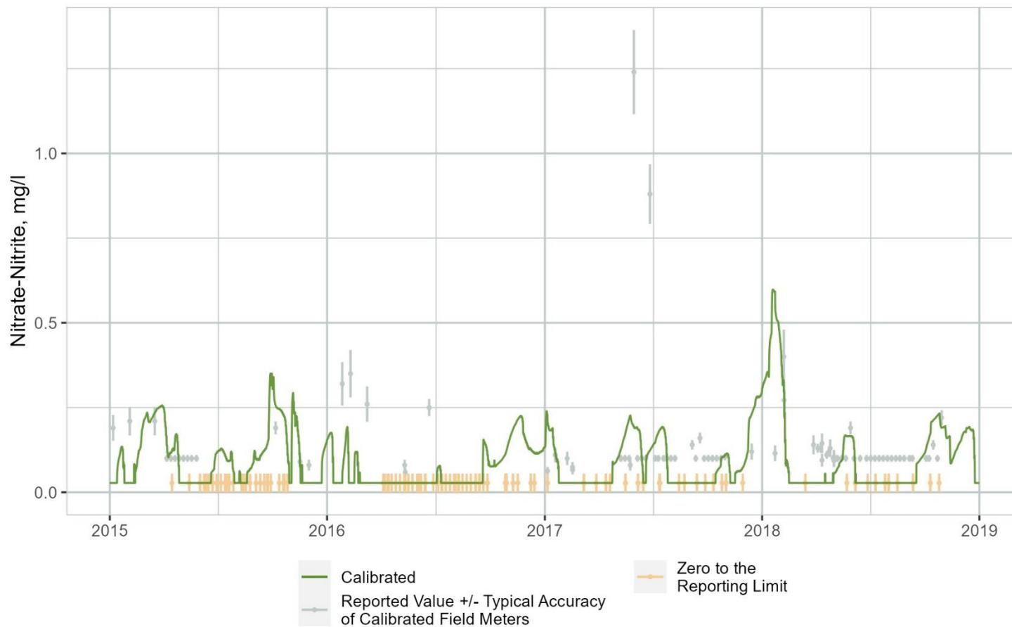
**Figure B-22. Time Series Comparison of WARMF Lake Simulated Nitrate plus Nitrite Concentrations to Observations Collected at the Downstream End of Segment 2**
