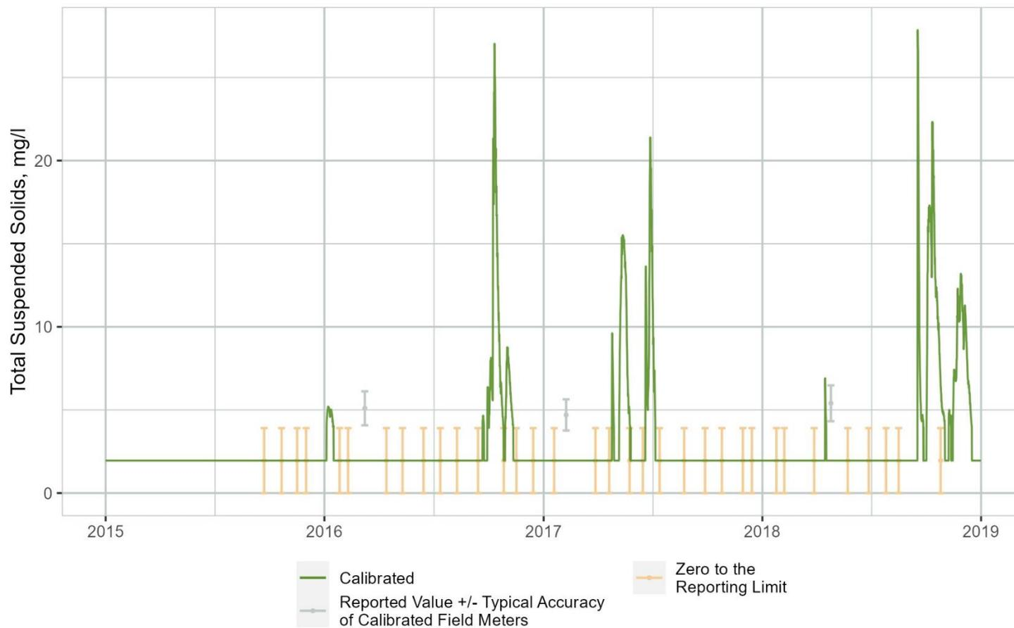
**Figure B-44. Time Series Comparison of WARMF Lake Simulated Total Suspended Sediment (TSS) Concentrations to Observations Collected at the Downstream End of Segment 6**
