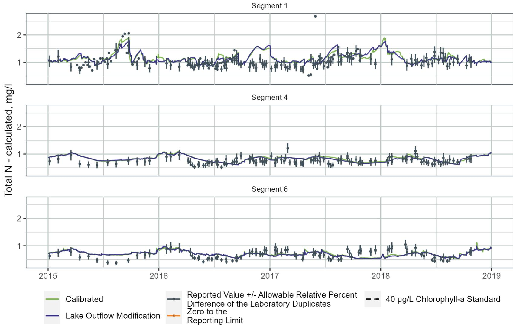
**Figure B-116. WARMF Lake Simulated Total Nitrogen Concentrations for the Calibrated Model Compared to the Dam Release Scenario with the Spillway Elevation Set to Normal Pool in Segment 1 (upper lake near Interstate 85), Segment 4 (middle lake near Highway 50), and Segment 6 (lower lake near the dam)**
