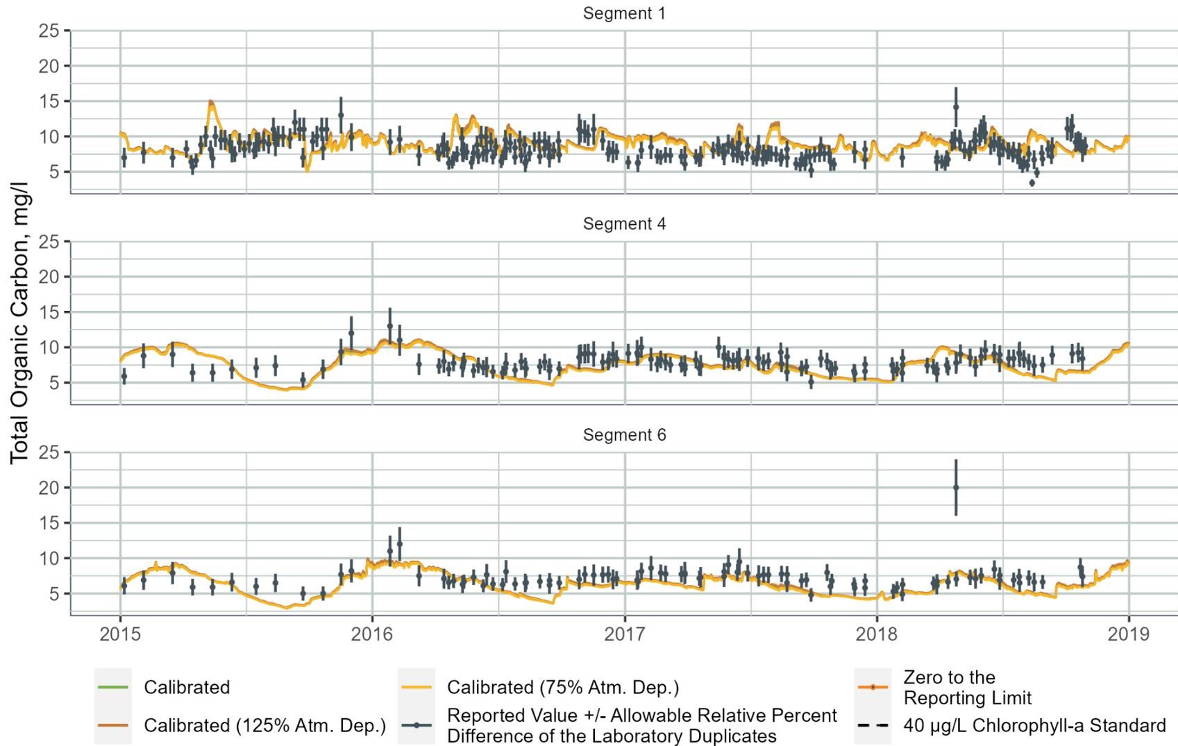
**Figure B-111. WARMF Lake Simulated Total Organic Carbon Concentrations for the Calibrated Model Compared to 25 Percent Increase or Decrease in Atmospheric Deposition of Total Nitrogen, Total Phosphorus, and Total Organic Carbon in Segment 1 (upper lake near Interstate 85), Segment 4 (middle lake near Highway 50), and Segment 6 (lower lake near the dam)**
