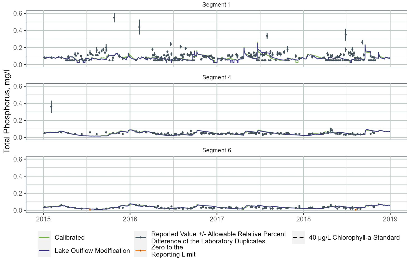
**Figure B-117. WARMF Lake Simulated Total Phosphorus Concentrations for the Calibrated Model Compared to the Dam Release Scenario with the Spillway Elevation Set to Normal Pool in Segment 1 (upper lake near Interstate 85), Segment 4 (middle lake near Highway 50), and Segment 6 (lower lake near the dam)**
