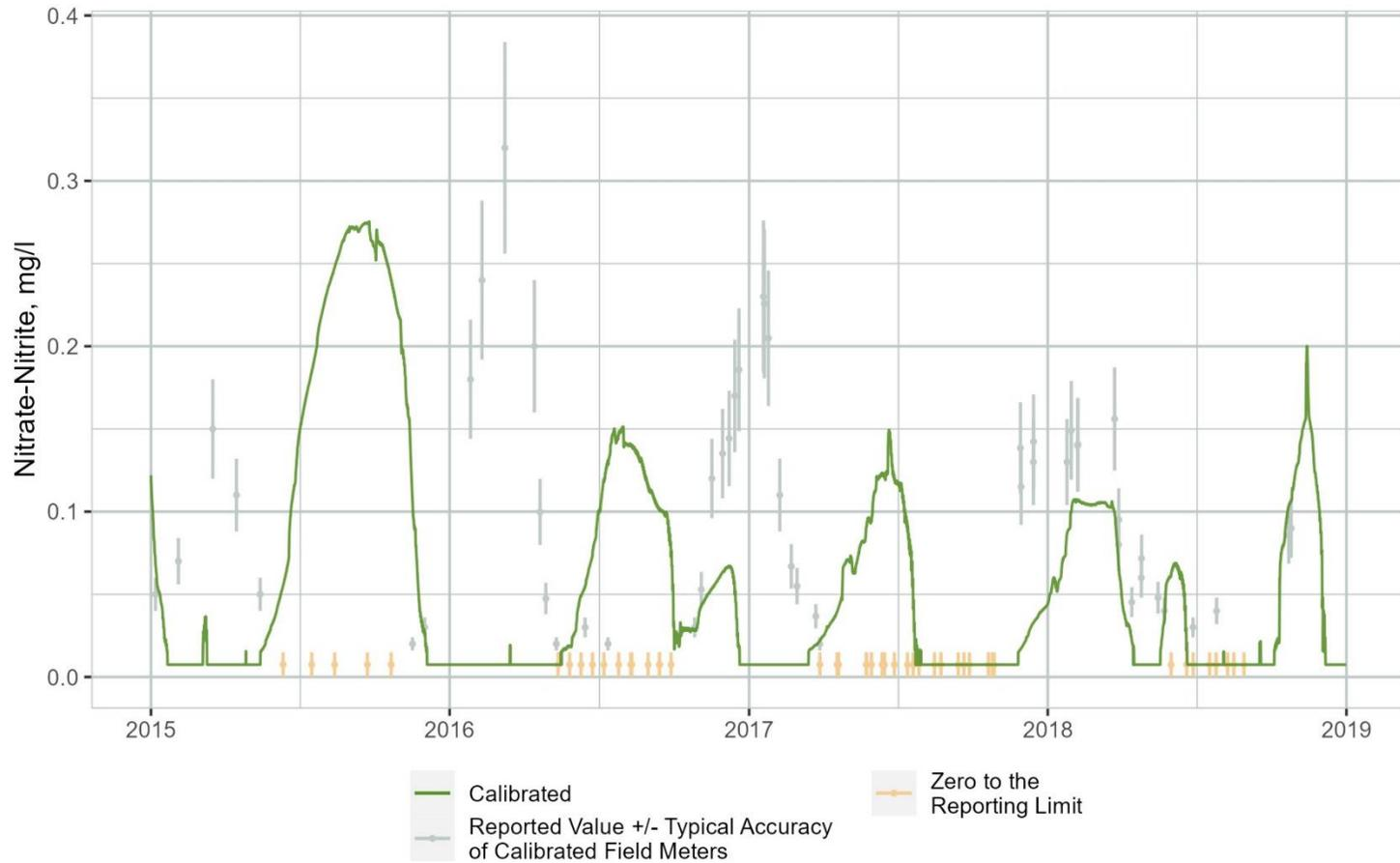
**Figure B-26. Time Series Comparison of WARMF Lake Simulated Nitrate plus Nitrite Concentrations to Observations Collected at the Downstream End of Segment 6**
