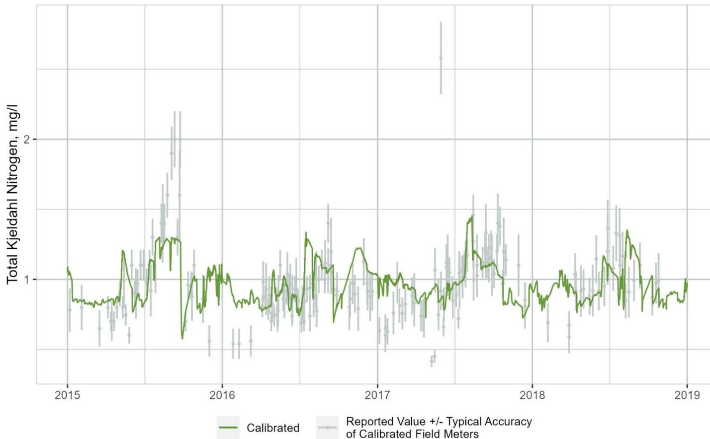
**Figure B-27. Time Series Comparison of WARMF Lake Simulated Total Kjeldahl Nitrogen (TKN) Concentrations to Observations Collected at the Downstream End of Segment 1**
