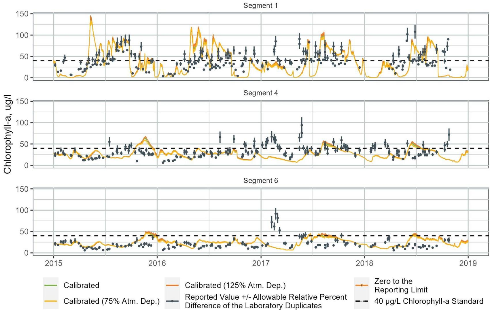
**Figure B-110. WARMF Lake Simulated Chlorophyll-a Concentrations for the Calibrated Model Compared to 25 Percent Increase or Decrease in Atmospheric Deposition of Total Nitrogen, Total Phosphorus, and Total Organic Carbon in Segment 1 (upper lake near Interstate 85), Segment 4 (middle lake near Highway 50), and Segment 6 (lower lake near the dam)**
