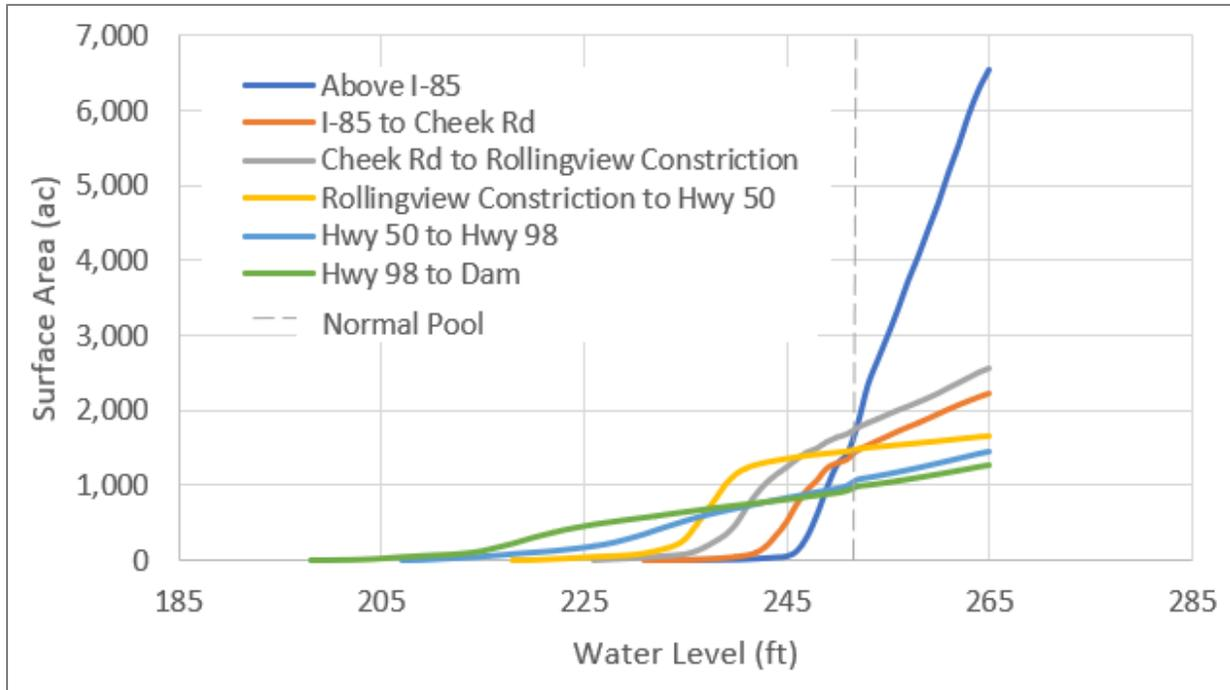
Figure B-5. Stage-Area Curve for the Mainstem Segments of Falls Lake
