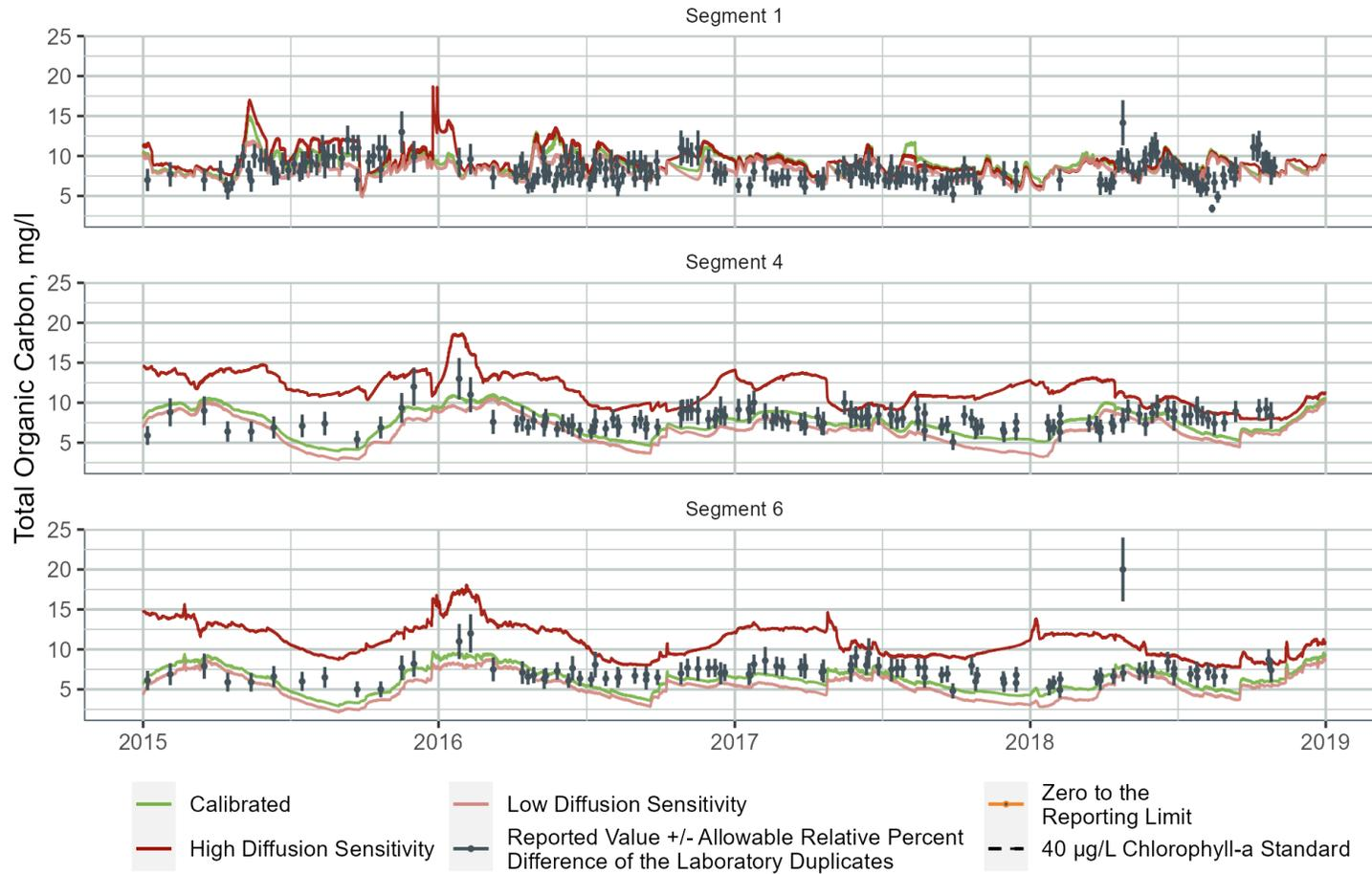
Figure B-84. TOC Sensitivity to Sediment Bed Diffusion Rate at Three WARMF Lake Segments
