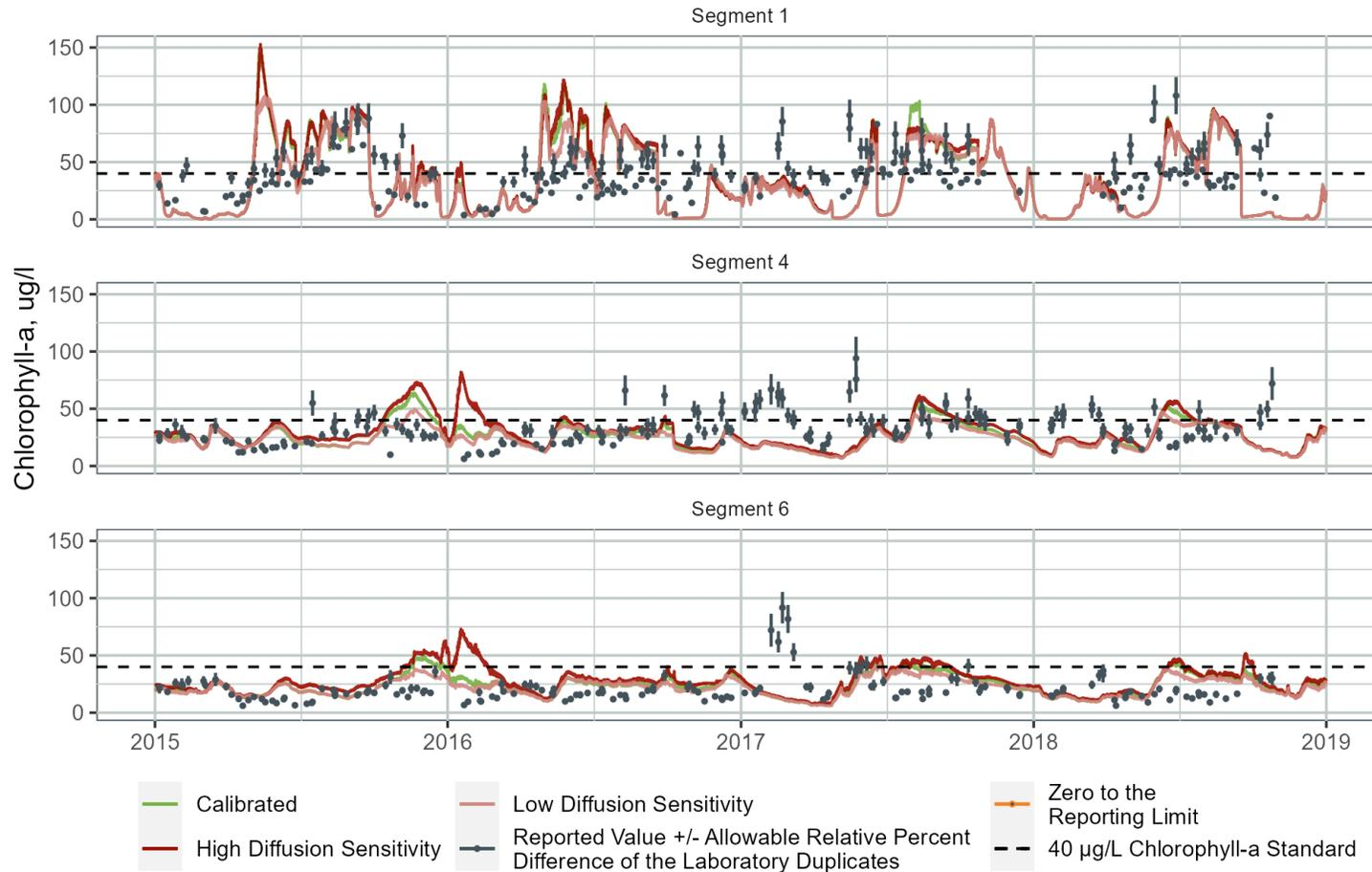
Figure B-87. Chlorophyll-a Sensitivity to Sediment Bed Diffusion Rate at Three WARMF Lake Segments
