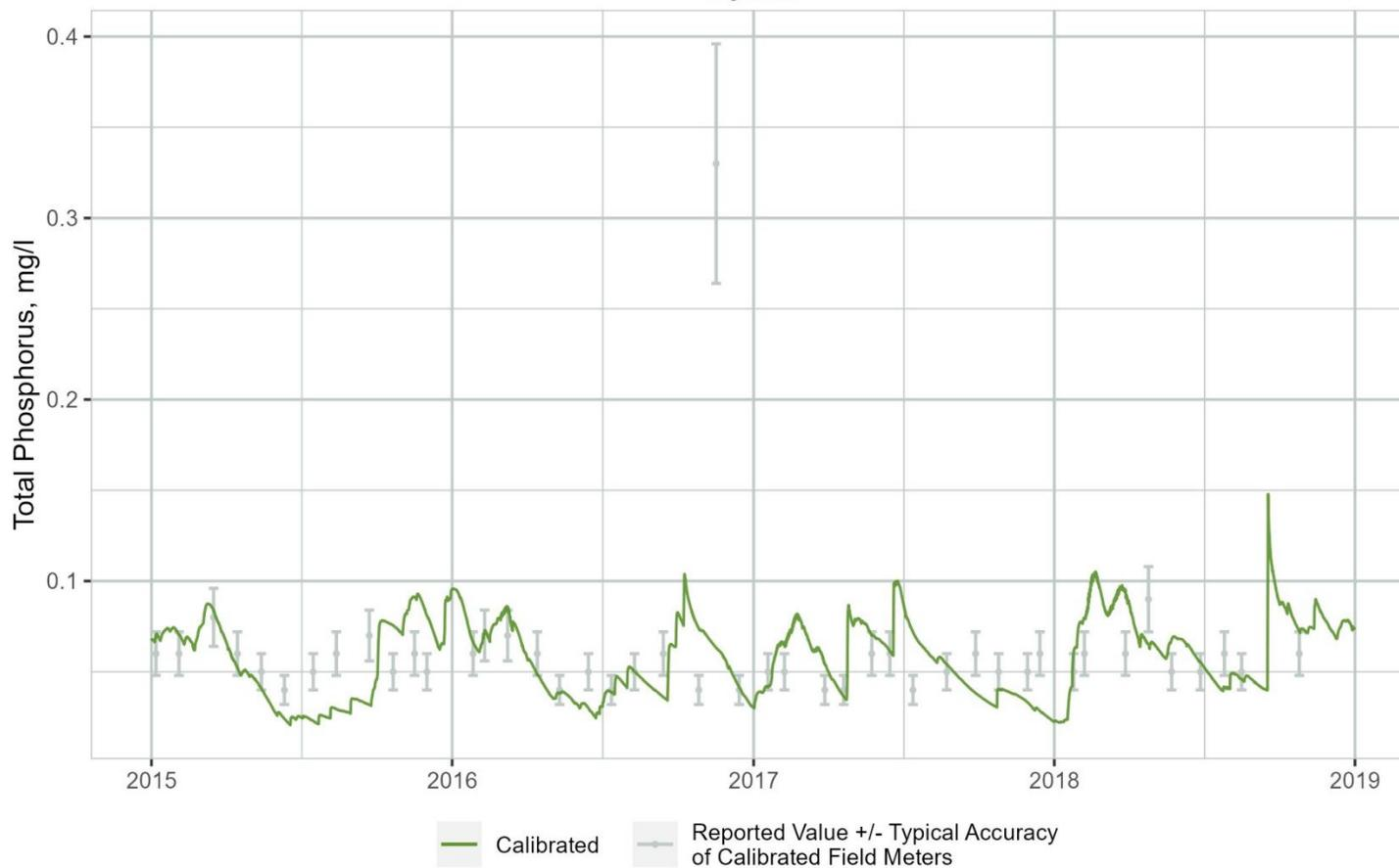
**Figure B-47. Time Series Comparison of WARMF Lake Simulated Total Phosphorus (TP) Concentrations to Observations Collected at the Downstream End of Segment 3**
