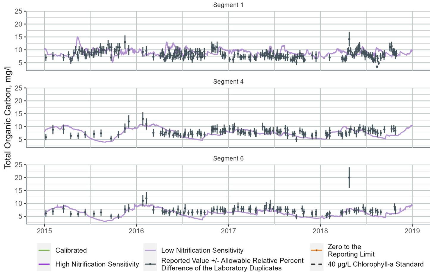
Figure B-92. TOC Sensitivity to Nitrification Rate at Three WARMF Lake Segments
