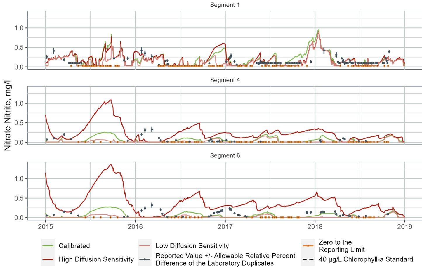
**Figure B-81. Nitrate plus Nitrite Sensitivity to Sediment Bed Diffusion Rate at Three WARMF Lake Segments**
