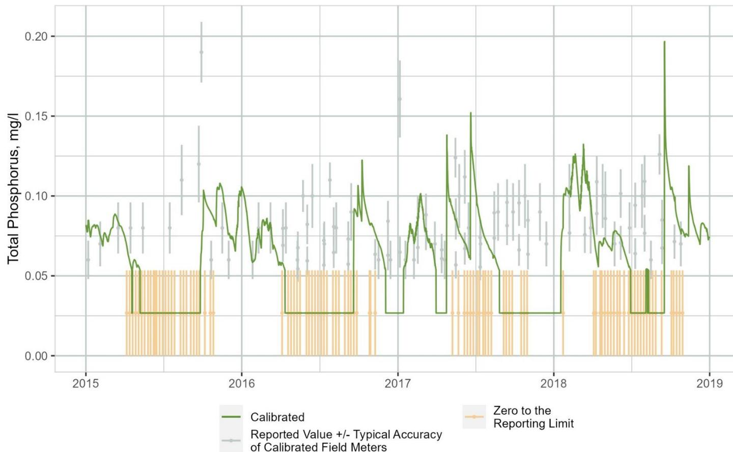
**Figure B-46. Time Series Comparison of WARMF Lake Simulated Total Phosphorus (TP) Concentrations to Observations Collected at the Downstream End of Segment 2**
