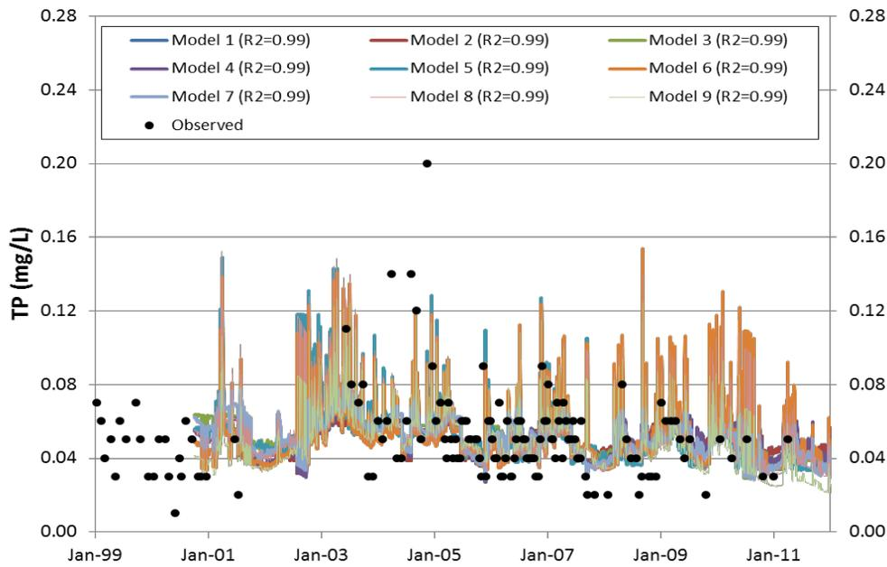
Figure A- 19 USGS LOADEST Predictions for TP (1999 to 2011) at Flat River below Lake Michie Dam Using Daily Average Flows
