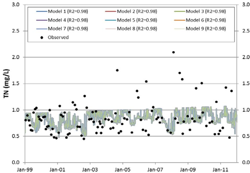
**Figure A- 25 USGS LOADEST Predictions for TN (1999 to 2011) at Little River below Little River Reservoir Using Daily Average Flows**
