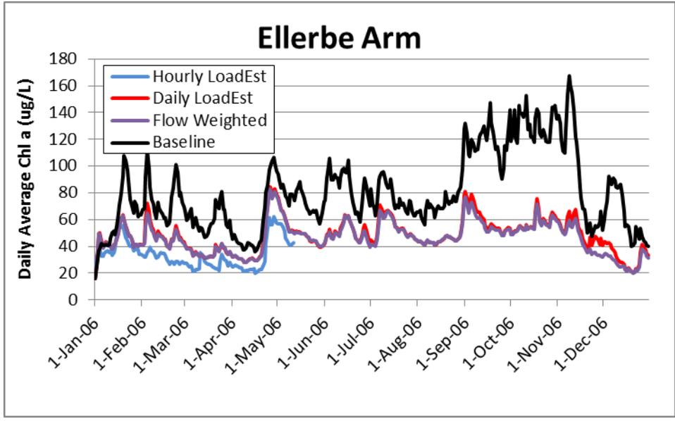
Figure 3-16 Simulated Chlorophyll a Concentrations in the Ellerbe Arm of Falls Lake Under Various EFDC Input Scenarios
