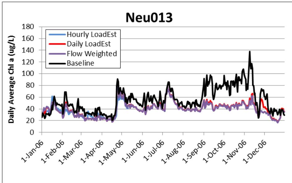
Figure 3-18 Simulated Chlorophyll a Concentrations Just Upstream of I-85 Under Various EFDC Input Scenarios
