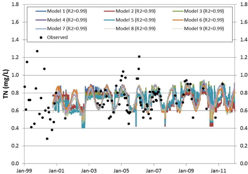
**Figure A- 21 USGS LOADEST Predictions for TN (1999 to 2011) at Flat River below Lake Michie Dam Using Daily Average Flows**
