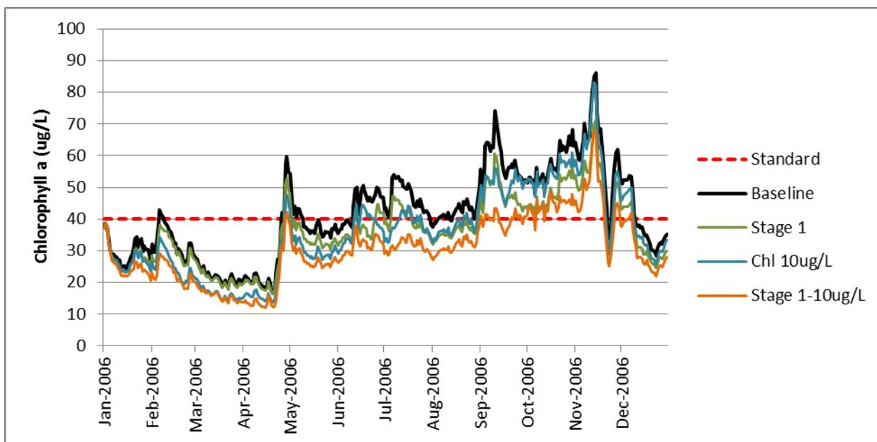
**Figure 3-2 Sensitivity of the EFDC Model to Tributary Chlorophyll a Assumptions for Baseline and Stage I Scenarios (at NEU013B)**
