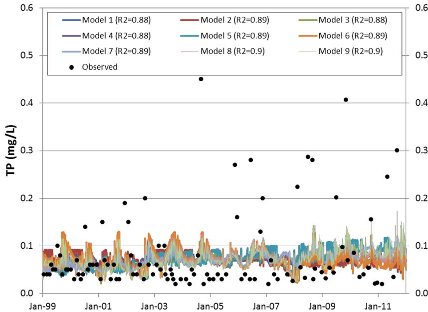
Figure A-23 USGS LOADEST Predictions for TP (1999 to 2011) at Little River below Little River Reservoir Using Daily Average Flows
