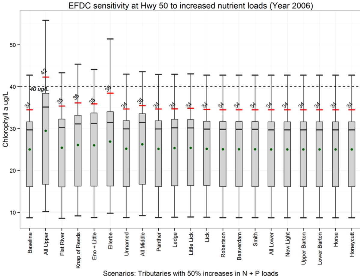
**Figure 3-5** Box Plots of Predicted Chlorophyll a Concentrations at Highway 50 Under Various Tributary Loading Scenarios
