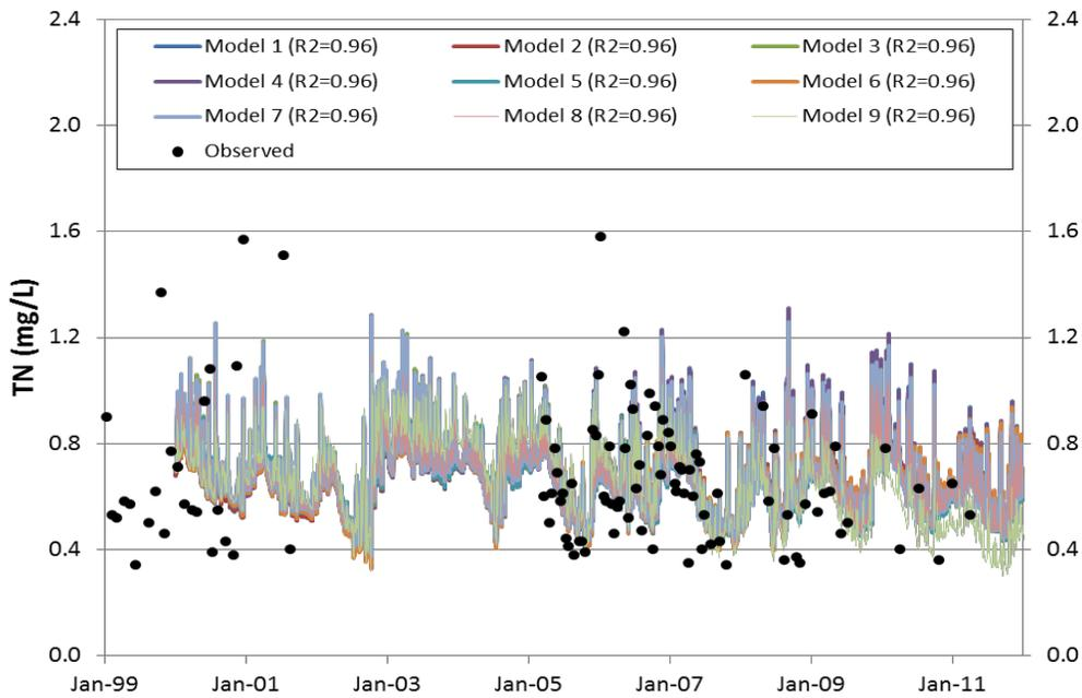
**Figure A- 17 USGS LOADEST Predictions for TN (2000 to 2011) at Eno River near Durham Using Daily Average Flows**
