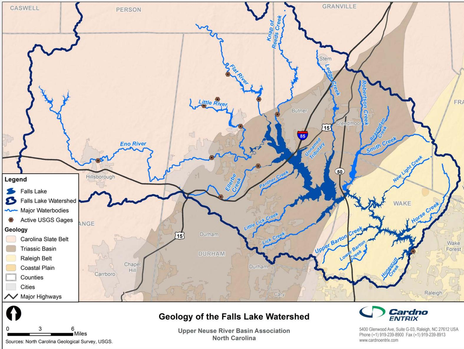
**Figure 1-1** Tributaries in the Falls Lake Watershed. The “upper” watershed and its tributaries are those located upstream of I-85. The “middle” watershed is that area between I-85 and Highway 50 (Creedmoor Road). The “lower” watershed is the area between Highway 50 and the Falls Lake Dam.
