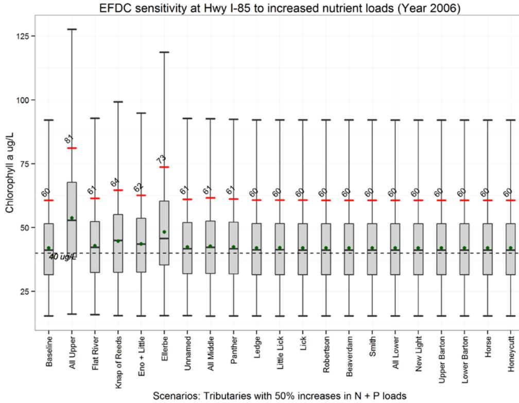
**Figure 3-3 Box Plots of Predicted Chlorophyll a Concentrations downstream of I-85 Under Various Tributary Loading Scenarios**
