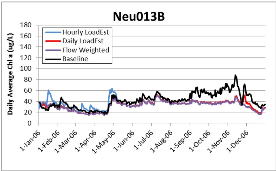
Figure 3-17 Simulated Chlorophyll a Concentrations Downstream of I-85 Under Various EFDC Input Scenarios
