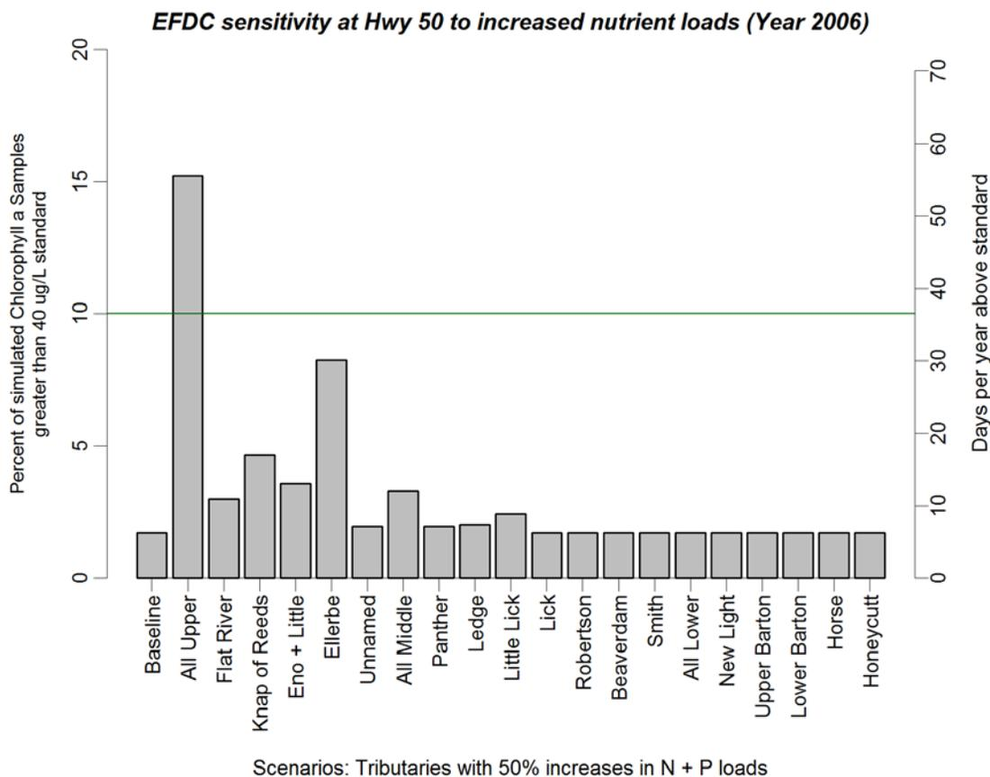
**Figure 3-6 Number of Days and Percent of Days When Predicted Chlorophyll a Concentrations at Highway 50 Exceeds the Water Quality Criterion Under Various Tributary Loading Scenarios**
