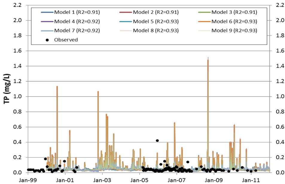
Figure A- 15 USGS LOADEST Predictions for TP (2000 to 2011) at Eno River near Durham Using Daily Average Flows
