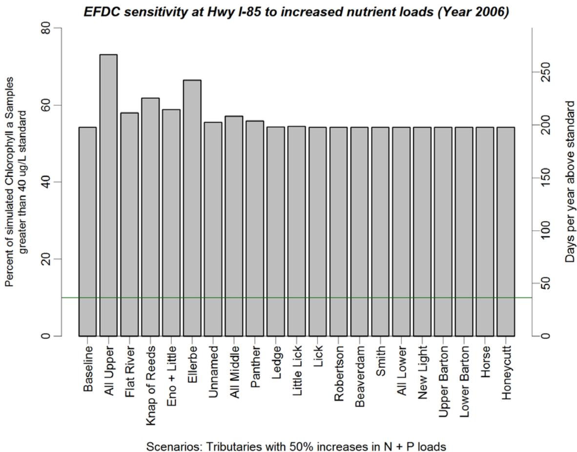
**Figure 3-4 Number of Days and Percent of Days When Predicted Chlorophyll a Concentrations downstream of I-85 Exceeds the Water Quality Criterion Under Various Tributary Loading Scenarios**
