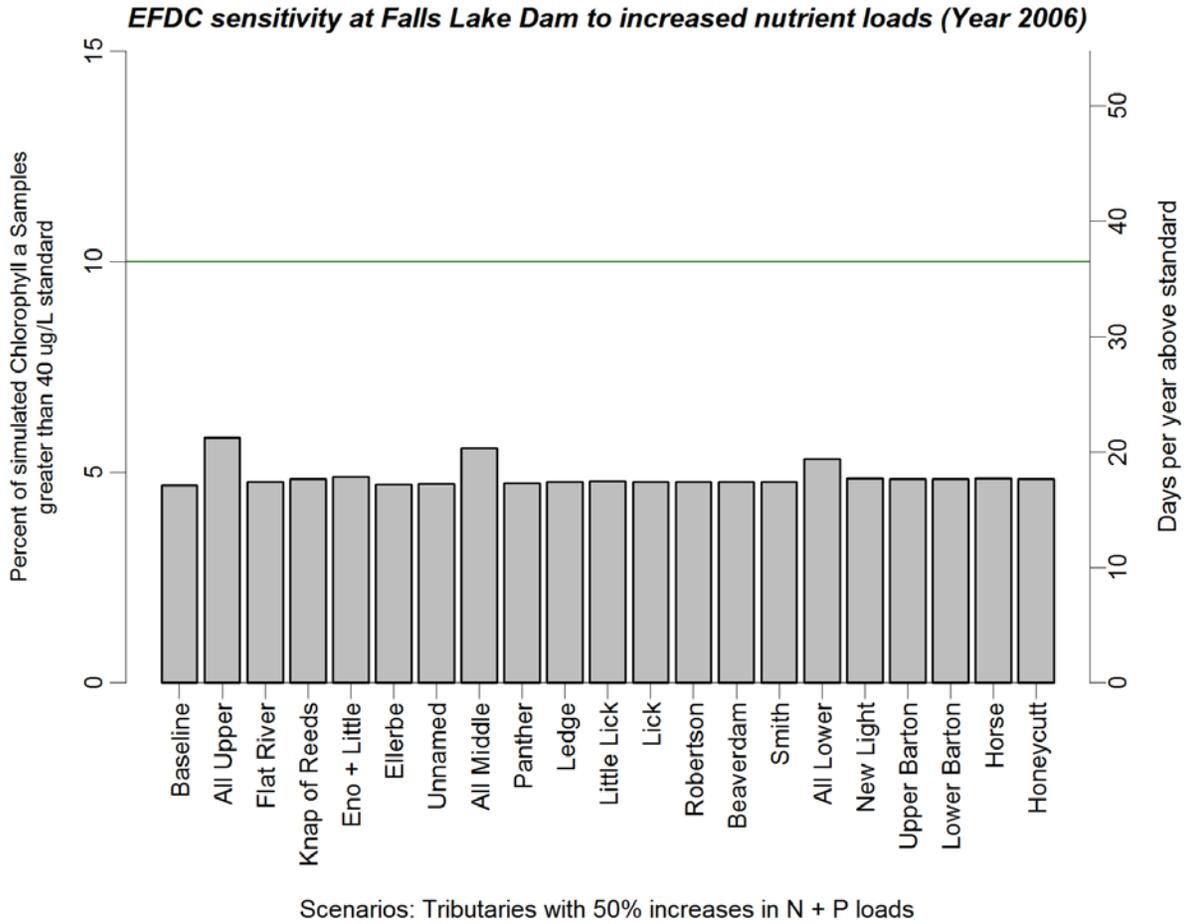
**Figure 3-8 Number of Days and Percent of Days When Predicted Chlorophyll a Concentrations at Falls Lake Dam Exceeds the Water Quality Criterion Under Various Tributary Loading Scenarios**
