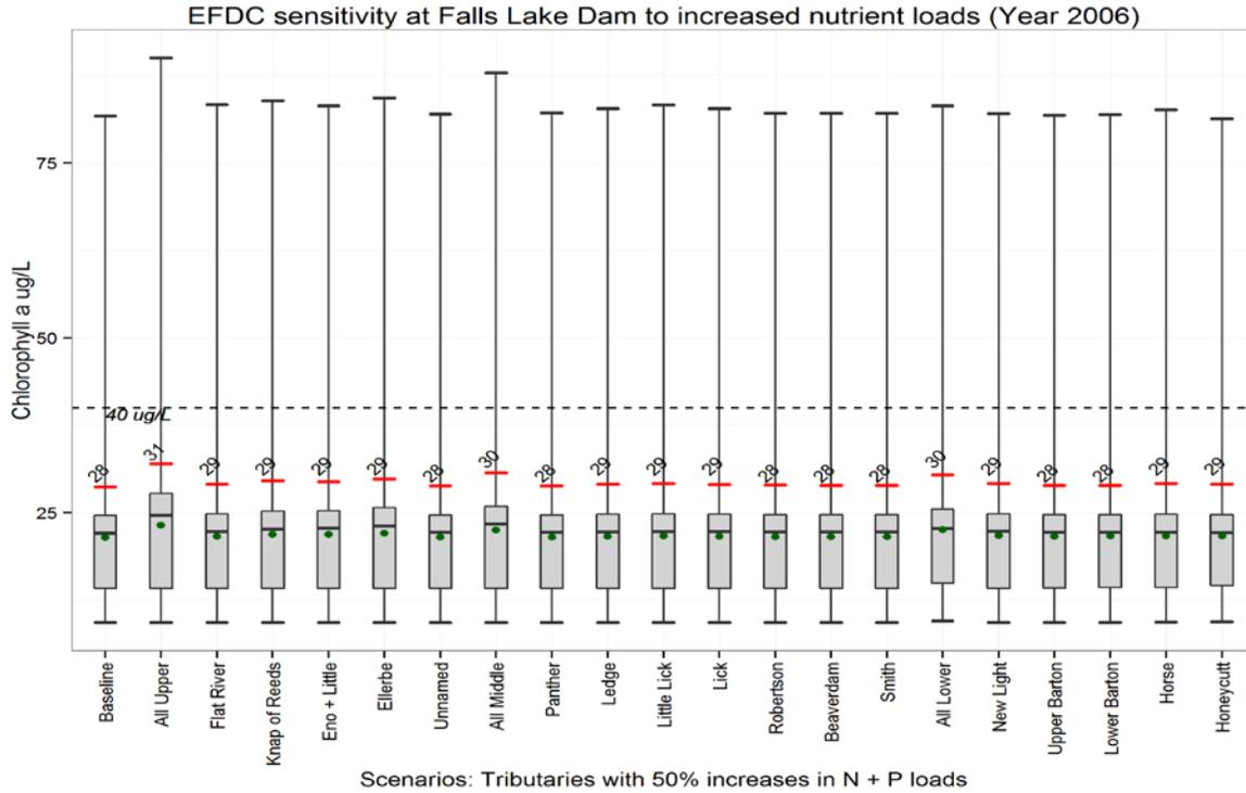
**Figure 3-7 Box Plots of Predicted Chlorophyll a Concentrations at the Falls Lake Dam Under Various Tributary Loading Scenarios**
